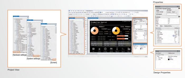
Configuration, from the entire project to individual screens, is consolidated into Project View, and individual settings into Properties.
