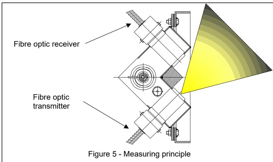
In order to keep the opacimeter away from the vibration and heat of the flue duct, two fibre optic cables handle the connection between the sensor and the processing electronics.
