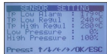
It is possible to adjust the measure of the sensor's low and high pressure sweeping air to adapt to the pressure present in the duct:
