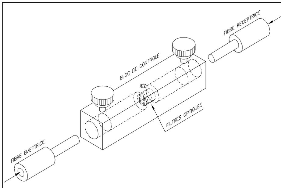
Figure 18 - Calibration control unit
