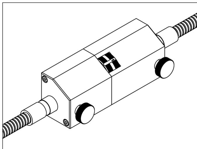
Calibration control block with 4 positions (3 control values and 1 null value position).
