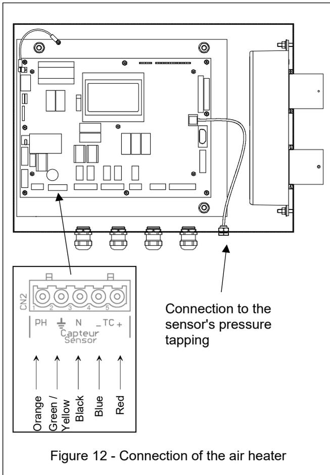
The air heater consists of a power resistor, supplied with 230V ~ (power 500W), and a temperature sensor (thermocouple type J).
