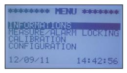
Pressing **OK** validates the chosen menu, pressing **ESC** cancels the operation and returns to normal display.
