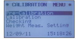
All operations of pre-calibration, calibration, weight measurements, etc. ..., must be performed on the values in the low scale of the device.
