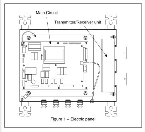
The ZFDM-4 electronics comprises 2 circuits :
