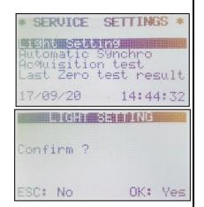
If a luminous flux adjustment is made, a calibration must be redone.
