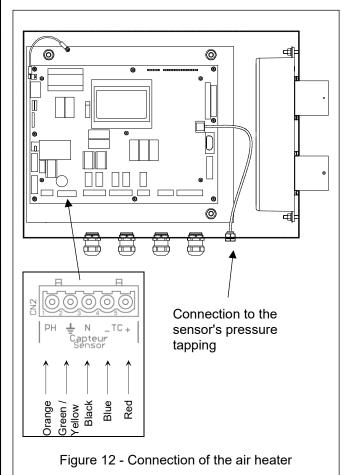
The air heater consists of a power resistor, supplied with 230V ~ (power 500W), and a temperature sensor (thermocouple type J).
