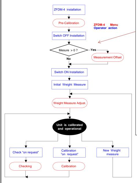
In situations of difficult measure (small diameter flue, flue lining reflective or light, etc ...), it may be a reflection of stray light induces an offset of measurement (measuring different from 0 without dust).
