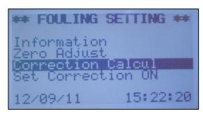
From the menu "FOULING SETTING", choose the sub-menu "CALCULATION CORRECTION" using the buttons  $\uparrow$  or  $\downarrow$  and confirm with OK.
