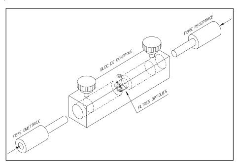
Figure 18 - Calibation control unit
