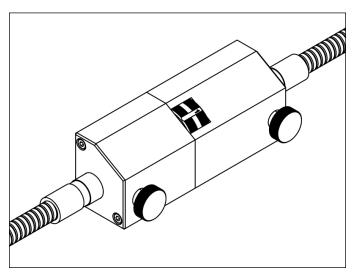
Calibration control block with 4 positions (3 control values and 1 null value position).
