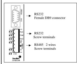
A serial link is available according to standard RS232 and RS485 standard (2 wires).
