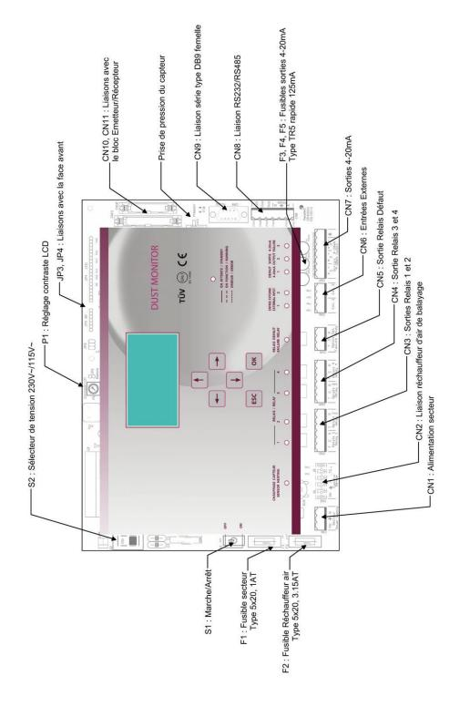
Figure 17 - Main printed circuit CP-4000
