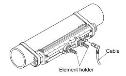
Stop turning the element holder where the transmitting surface contacts the surface of pipe, and thus the element holder will not rotate. Do not turn it excessively.
