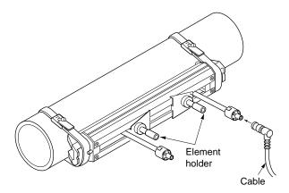
Stop turning the element holder where the transmitting surface contacts the surface of pipe, and thus the element holder will not rotate. Do not turn it excessively.
