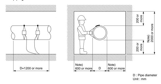
Fig. 5-1 Necessary space for the detector mounting position
