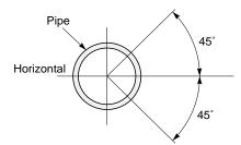
(2) Avoid installing the sensor on a deformed portion of pipe or welded portion of pipe, or on flange.
