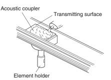
Turn the element holder counterclockwise to return the sensor.
