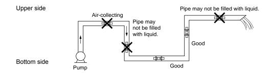
(2) Where a horizontal pipe is used, install the sensor within ±45° from the horizontal plane. Otherwise, the measurement could be impossible if bubbles stay in the upper part of piping or if deposits are accumulated in the lower part of piping. In case of vertical piping, the detector may be mounted at any position on its periphery provided that the flow is upward.
