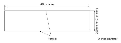
(2) Draw a line that intersects with the long sides at right angles at a place about 100 mm from one end.
