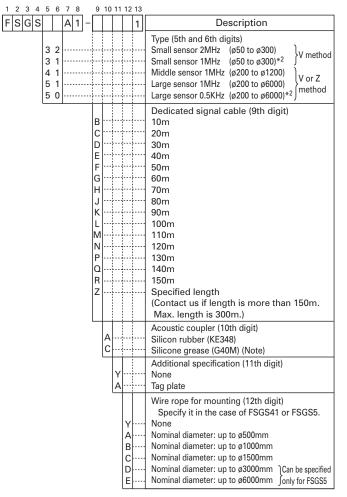
\*2: For aging pipes, cast iron pipes or mortar-lined pipes that interrupts the propagation of ultrasonic signals, select FSGS31 or FSGS50.
