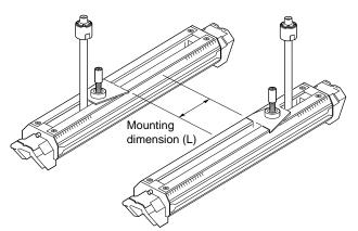
(3) Spread acoustic coupler over the whole transmitting surface of the sensor.
