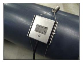
Make sure that the matching mark on the sensor is aligned with the marking line. In addition, make the transmitting direction marks of sensors face each other.
