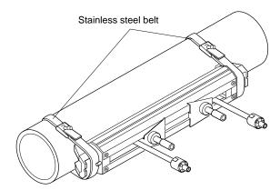
(4) Make sure that the sensor is mounted in parallel with the piping and that the mounting position is correct. Then, turn the element holder clockwise until the sensor is firmly fitted to the piping.
