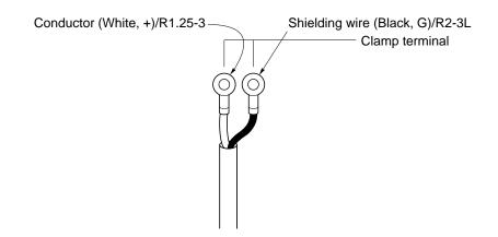
Note) When cutting the coaxial cable, make sure that the upstream side and the downstream side are the same in length.
