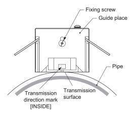
Loosen the guide plate fixing screw and slide the guide plate until its edge and transmitting surface touch the surface of pipe. Tighten the retaining screw.
