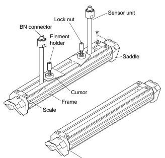
Guide rail for high temperature sensor
