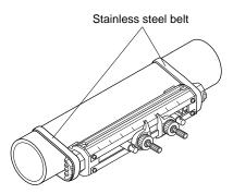
(4) Make sure that the sensor is mounted in parallel with the piping and that the mounting position is correct. Then, turn the element holder clockwise until the sensor is firmly fitted to the piping.
