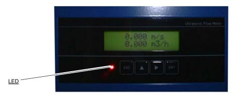
4.1.2. Flow transmitter : FSV···H (IP67) display/setting unit
