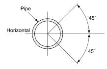
(3) Avoid installing the sensor on a deformed portion of pipe or welded portion of pipe, or on flange.
