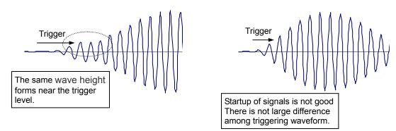
Cause of the poor startup signals
