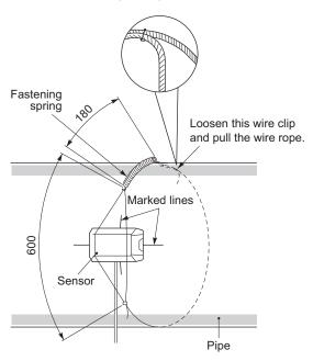
Loosen the wire clip and pull the wire rope until the overall length of fastening spring approximates 180mm. Then tighten the wire clip. (The fastening spring has a free length of 110mm.) Remove the sensor with the wire rope fixed in place.
