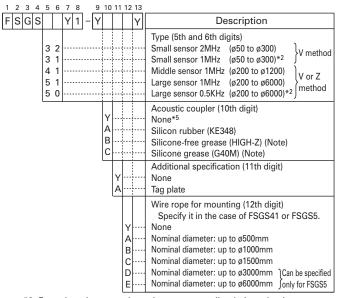
\*2: For aging pipes, cast iron pipes or mortar-lined pipes that interrupts the propagation of ultrasonic signals, select FSGS31 or FSGS50.
