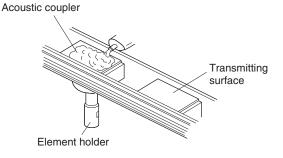
Turn the element holder counterclockwise to return the sensor.
