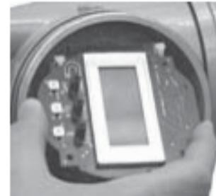
7. Push card in, between holding clips. Lower card back into position, and attach card with screws and washers.
