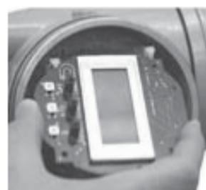
4. Gently pull card down and out from between holding clips.
