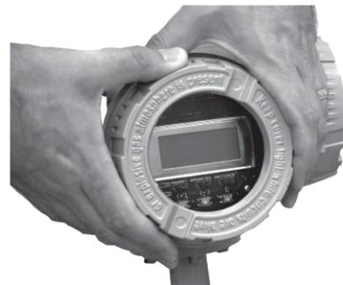
2. Remove the 2 display card screws and washers.
