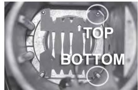
11. When placing display card back into PCB Display, verify mark and red stripe are aligned with Number 1.
