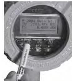
The other method involves removing the display chamber cover and manipulating the +, - and E push buttons to view and change settings and program desired meter functions and settings.
