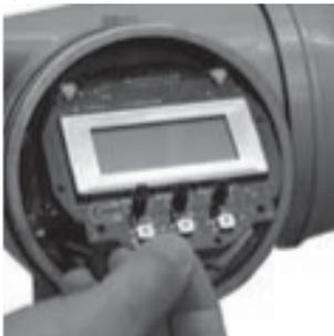
4. Gently pull card down and out from between holding clips.
