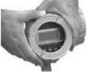
2. Remove the 2 card screws and washers. (NOTE: Use a split screwdriver to prevent dropping screw into enclosure.)
