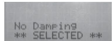
20. And this type of screen shows for 2 seconds when Damping Factor time is selected.
