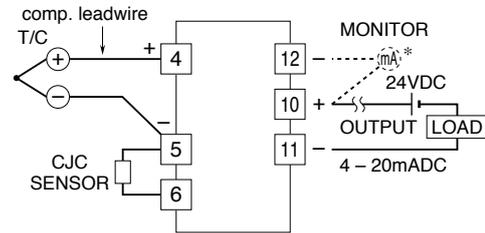
\*DC ammeter's internal resistance 10 ohms max.
