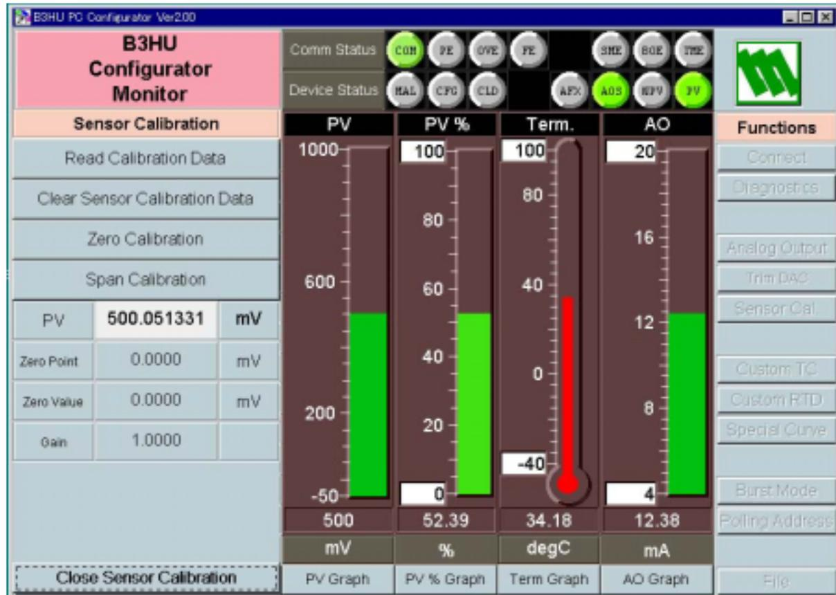
The present measured value is indicated in the middle. Refer to this value when calibrating the sensor. It takes 5 or 6 seconds for the calibration result affects the measured value on the display.
