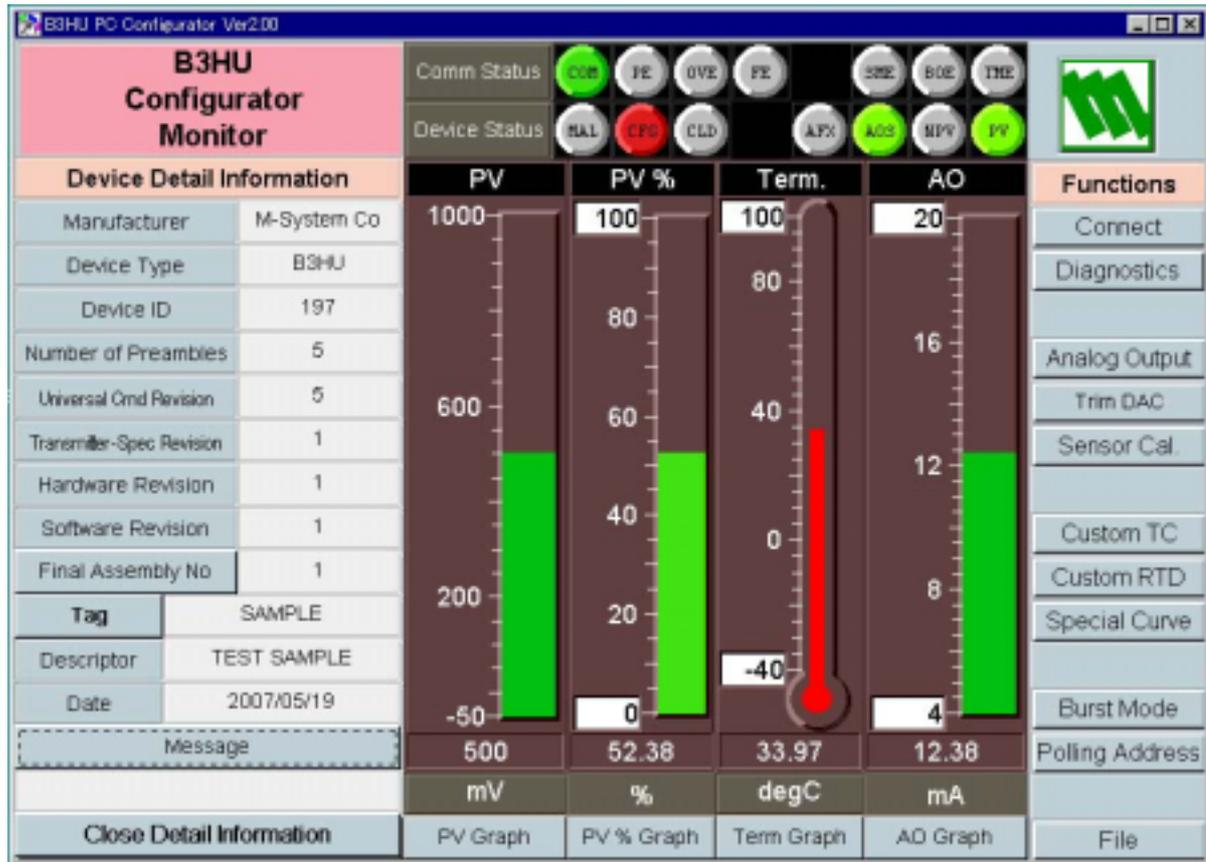
The menu shows the following items: Manufacturer, Device Type, Device ID, Number of Preambles, Universal Command Revision, Transmitter-Specific Revision, Hardware Revision, Software Revision, Final Assembly No., Tag, Descriptor, Date and Message.
