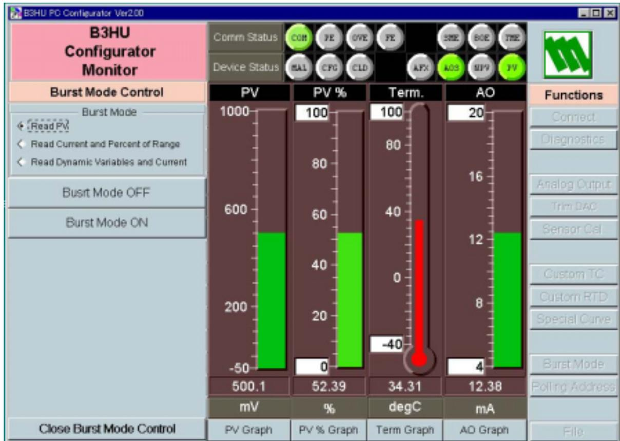
[Burst Mode ON] Enables the burst mode as specified in the menu.
