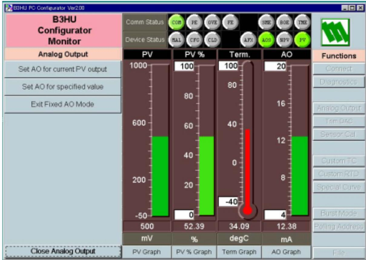
[Set AO for current PV output] The output current is held at the current value.
