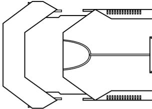
**Caution:** DO NOT PULL beyond where the housing cover is latched. The plastic housing may be damaged.
