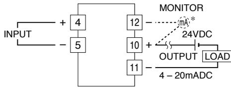
\*DC ammeter's internal resistance 10 ohms max.
