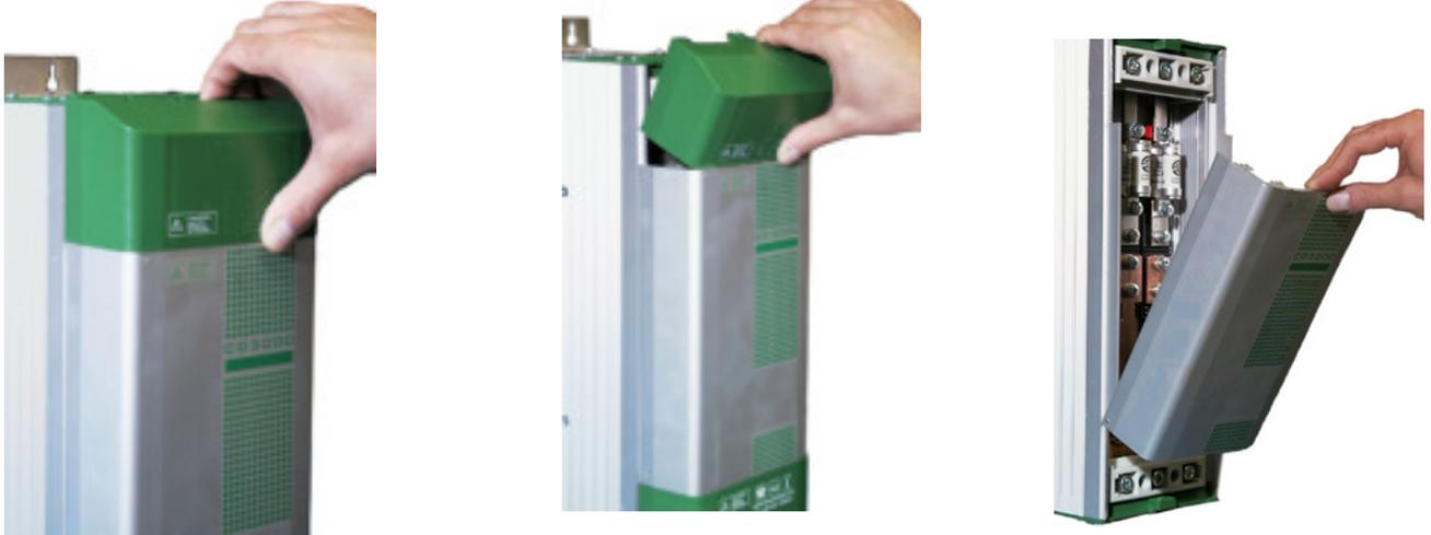
For S9 size, you must open the cover to configure the unit and to view the fuses
