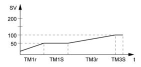
• The SV limit function (SV-h, SV-L) is in effect while ramp/soak is running.
