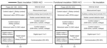
insulation class for equipment meets usage requirements.
