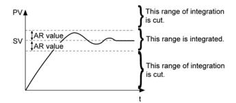
[Setting example] Changing the anti-reset windup to 500°C
