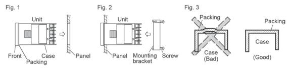
Mounting on vertical plane (in horizontal position)
