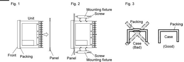
Mounting on vertical plane (in horizontal position)
