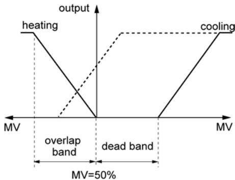
"db" is called dead band when the value is positive, and overlap band when the value is negative.
