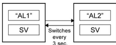
[Setting example] Setting to display only the alarm status during an alarm \_\_\_\_\_
