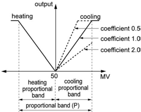
Cooling proportional band is set after the optimal value for heating proportional band is set.
