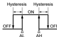
[Setting example ] Setting the Alarm 1 hysteresis to 5°C, delay time to 30, and delay time unit to seconds
