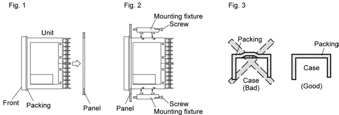
Mounting on vertical plane (in horizontal position)
