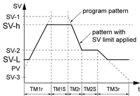
[Setting example] Setting SV1, ramp time, and soak time for step1 \_\_\_\_\_
