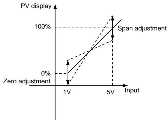
[Setting example] Adjusting zero and span in PV display
