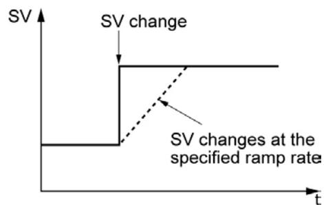
[Setting example] Setting the ramp SV incline to 10°C/min, and decline to 5°C/min \_\_\_\_\_
