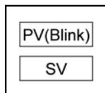
Setting 3: The alarm status is only displayed when an alarm or alarms occur. PV is not displayed.
