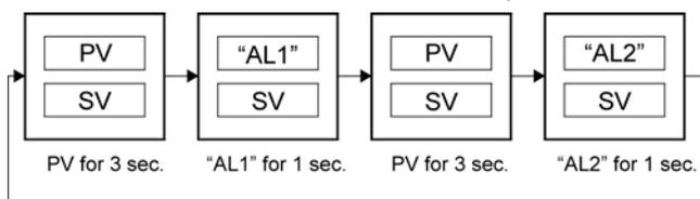
Setting 2: Blinking PV is displayed when an alarm or alarms occur.
