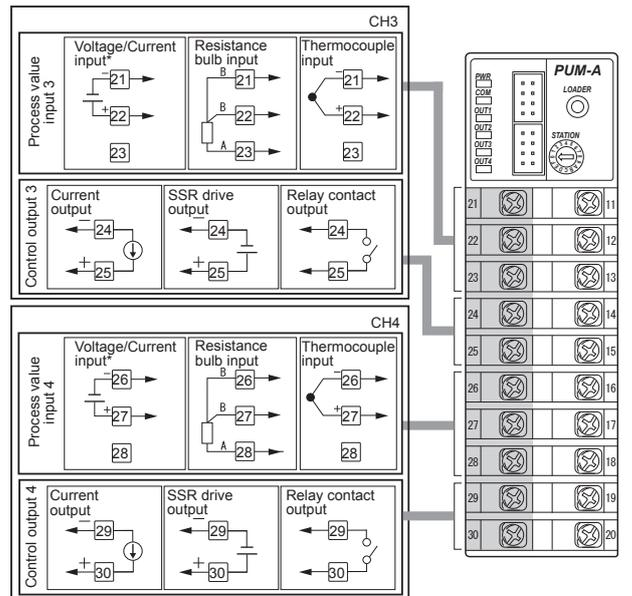
\*In case of current input, attach I/V unit which comes with the controller to the voltage input terminal.
