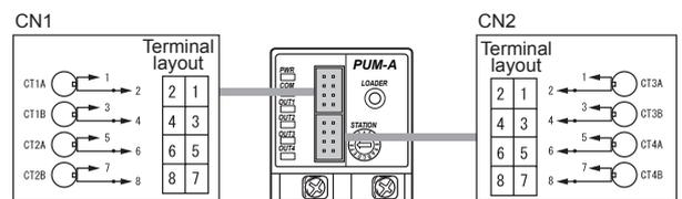
\*Pin No. 2, 4, 6, 8 of CN1 and CN2 are connected inside the equipment.
