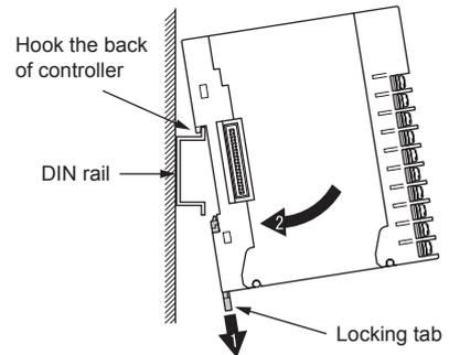
3. Push up the locking tab to fasten the controller onto DIN rail.
