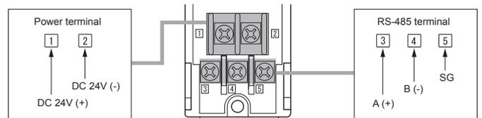
All connected controllers are connected to power supply and RS-485 via side connectors if one of controllers is directly connected to them.
