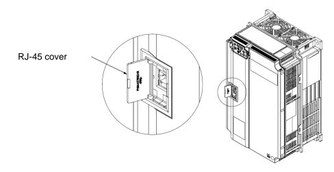
Figure 2.4-1 (b) Connection of the RS-485 Communication Cable
