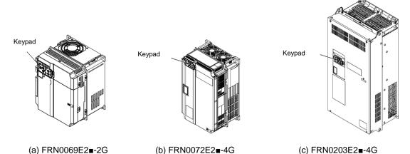
Figure 2.3-1 Attaching the Keypad to the Inverter Main Body
