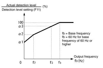
Characteristics diagram of motor cooling system
