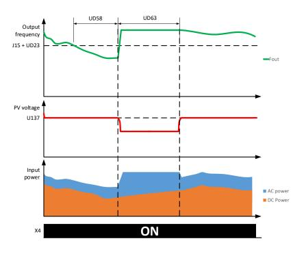
Note As explained in this section, when U136 is set to certain values, the sleep function might be deactivated. As the AC power is activated and there might be no worries about the available power, sleep function would be reached in case of pressure control or the like.
