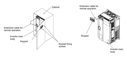
Figure 2.3-2 Attaching the Keypad on the Cabinet
