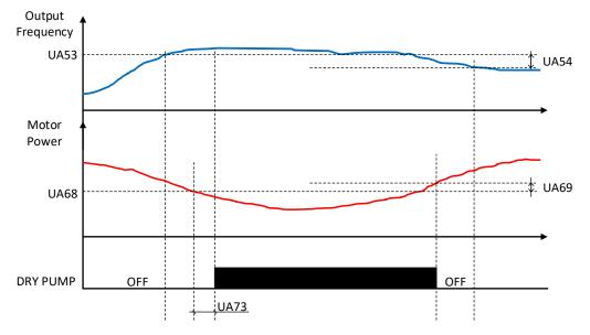
Function code U124 is used to enable the alarm "OH2" in case that dry pump state is detected, by setting this function code to 1.00.
