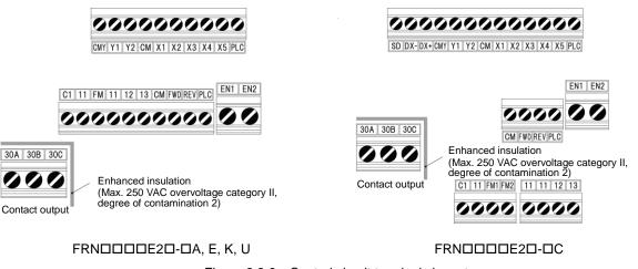
Figure 2.2-8 Control circuit terminals layout
