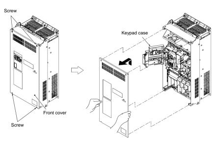
Tightening torque: 1.8 N·m(15.9 lb-in) (M4) 3.5 N·m(31.0 lb-in) (M5)
