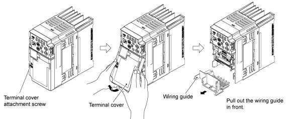
Figure 2.2-1 Removal of the Terminal Cover and the Wiring Guide (for FRN0006E2S-2D)
