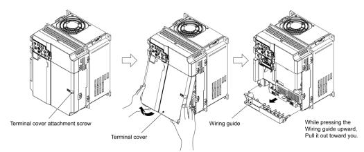
Figure 2.2-2 Removal of the Terminal Cover and the Wiring Guide (for FRN0069E2=-2□)
