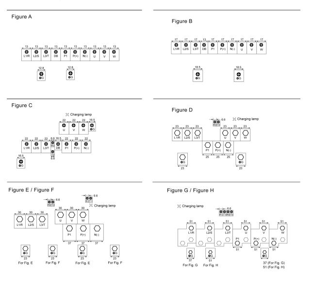
Figure 2.2-7 Main circuit terminals layout
