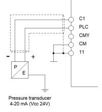
The maximum scale of the pressure transducer can be set in UJ18, parameter. This will scale the meaning of the pressure transducer 4-20mA, as well as the PID setpoint in parameter U122.
