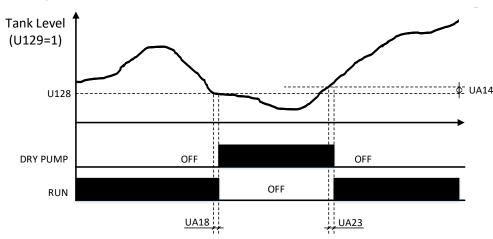
Dry pump detection function when using an analogue input
