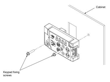
Figure 2.3-7 Attachment of the Keypad
