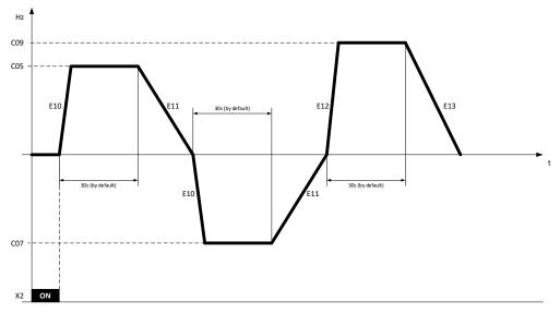
The antijam pattern can be set with the "Pattern operation" stages 1-6, according to the figure above. Please check FRENIC Ace users' manual for further information on the pattern operation settings.
