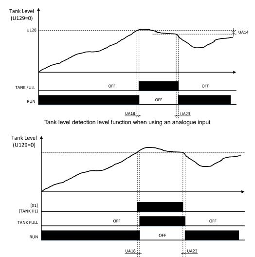
Tank level detection level function when using a digital input
