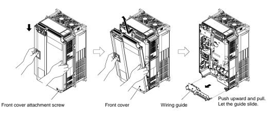
Figure 2.2-3 Removal of the Front Cover and the Wiring Guide (for FRN0072E2=-4□)
