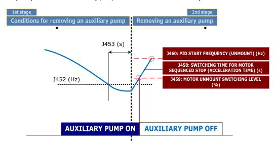
Figure 2.7: Disconnection of an auxiliary pump
