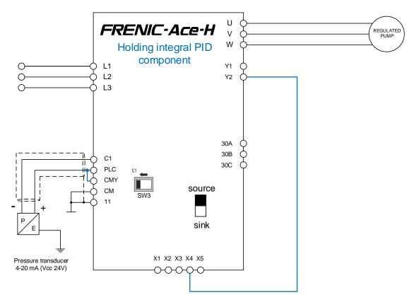
Figure 5.3: Pump control schematic for holding PID Integral component when pump is in sleep mode
