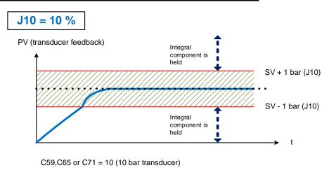
Figure 5.4: PID behaviour when function J114 is used.
