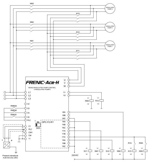
Figure 4.2: Schematics of multi-regulated pump control with 3 regulated pumps (Using OPC-F2-RY)
