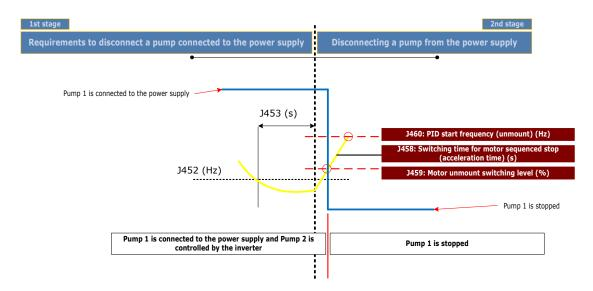
Figure 4.6: Increase of the pump's speed to disconnect the pump from the main supply
