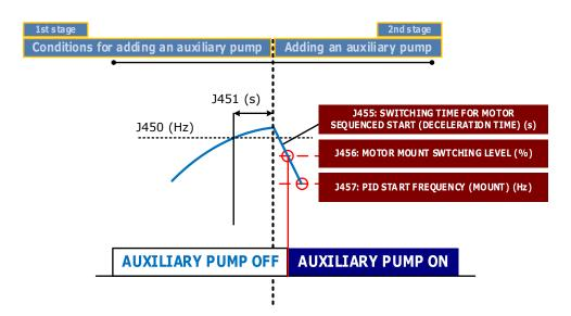
Figure 2.6: Auxiliary pump's connection
