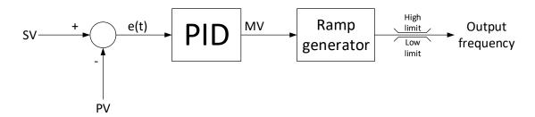
Figure 1.3: PID control schematics inside the inverter
