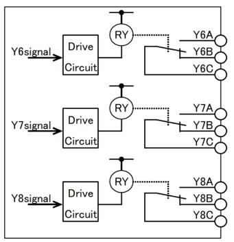
Figure 8.1 Internal Diagram OPC-F2-RY
