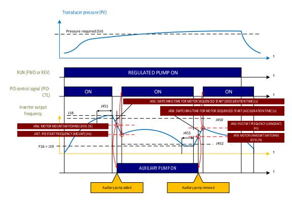
Figure 2.5: Speed pattern with mono-regulated pump control. The Auxiliary pump is connected and disconnected
