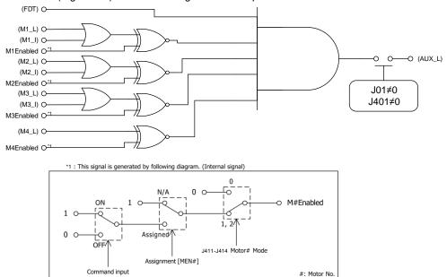
Figure 3.3: Additional pump function logic block diagram
