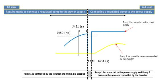
Figure 4.5: Connection of a regulated pump to the commercial power supply.
