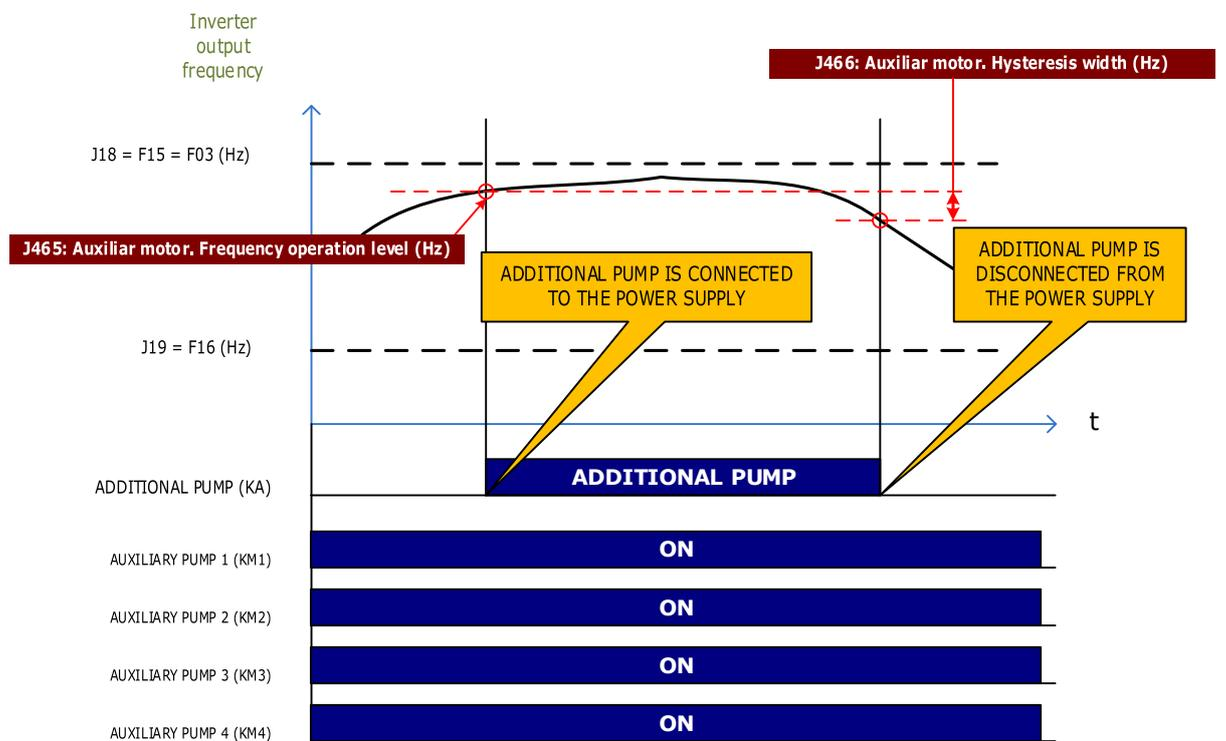
Figure 3.2: Additional pump’s connection/disconnection diagram if all the auxiliary pumps are enabled
