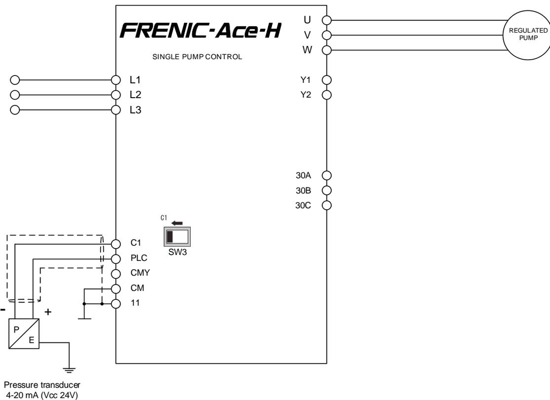
Figure 1.1: control schematic for 1 pump only
