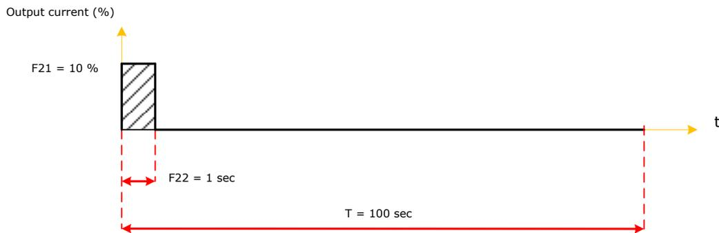
Figure 5.2: Output current when Dew Condensation prevention function is enabled
