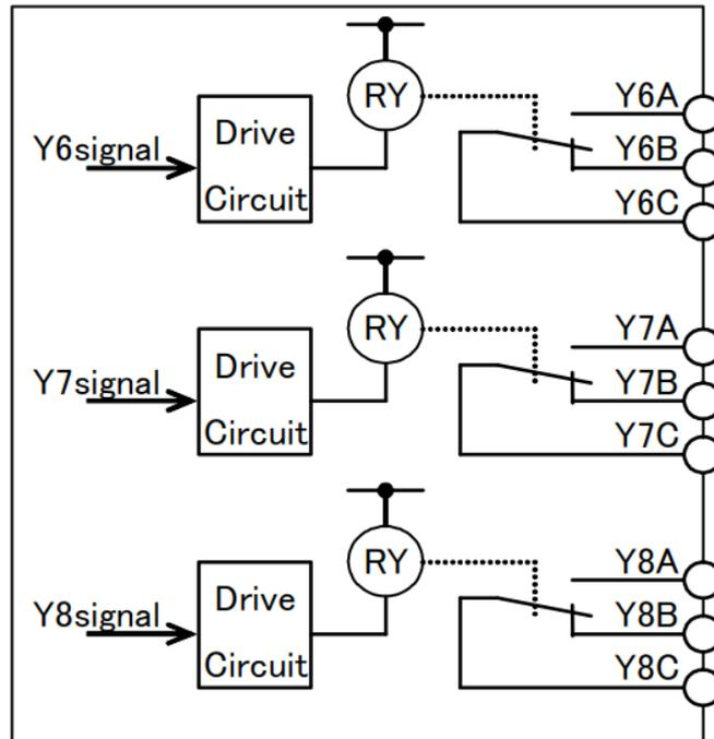
Figure 8.1 Internal Diagram OPC-F2-RY
