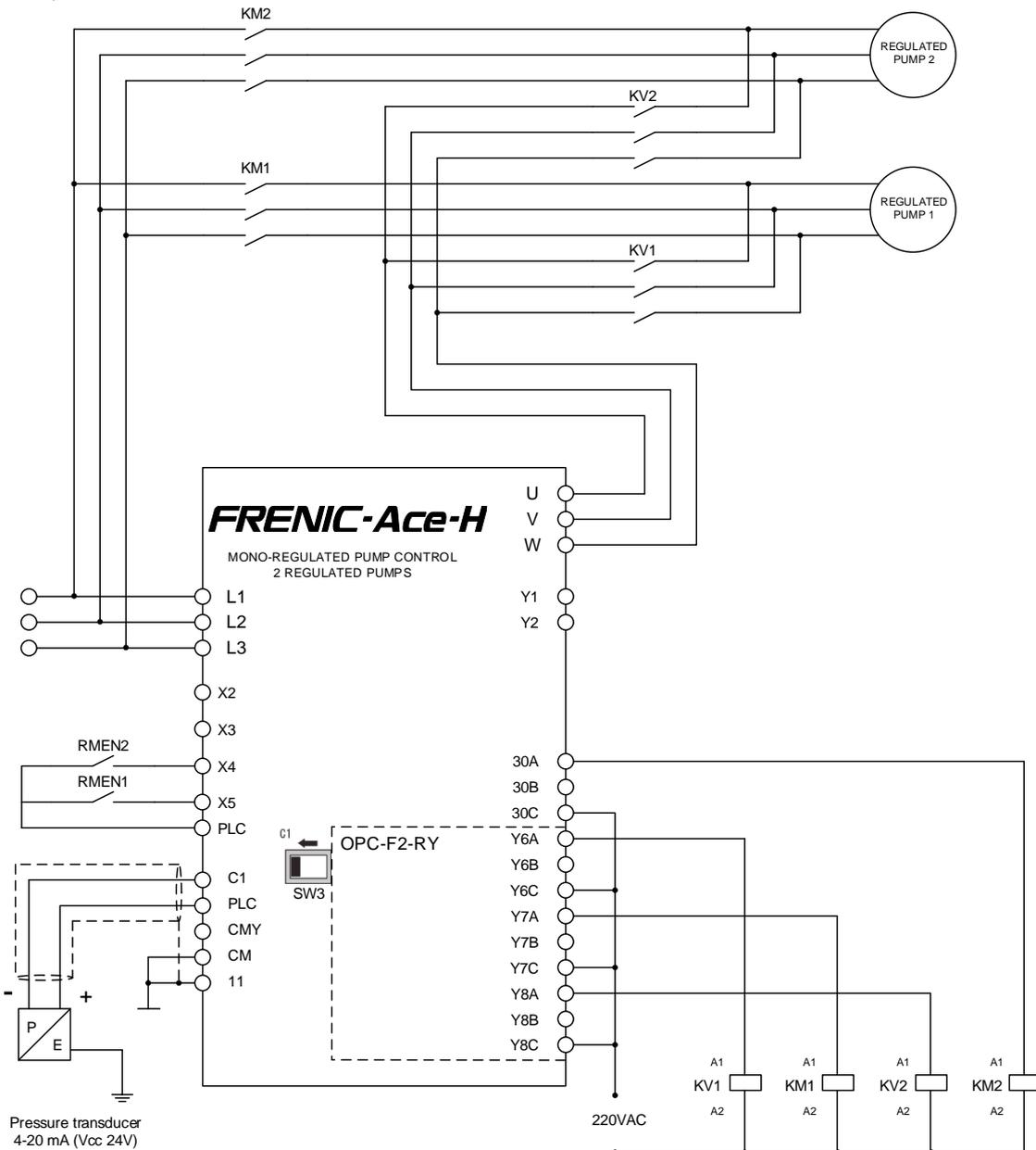
Figure 4.1: Schematics of multi-regulated pump control with 2 regulated pumps (Using OPC-F2-RY)
