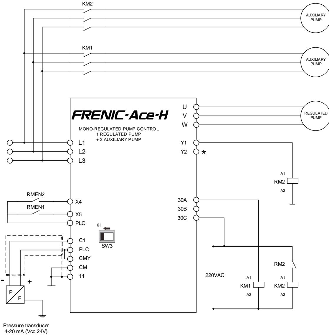
Figure 2.2: Schematic of a mono-regulated pump control with 1 regulated pump + 2 auxiliary pumps with external relays.
