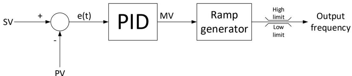
Figure 1.3: PID control schematics inside the inverter
