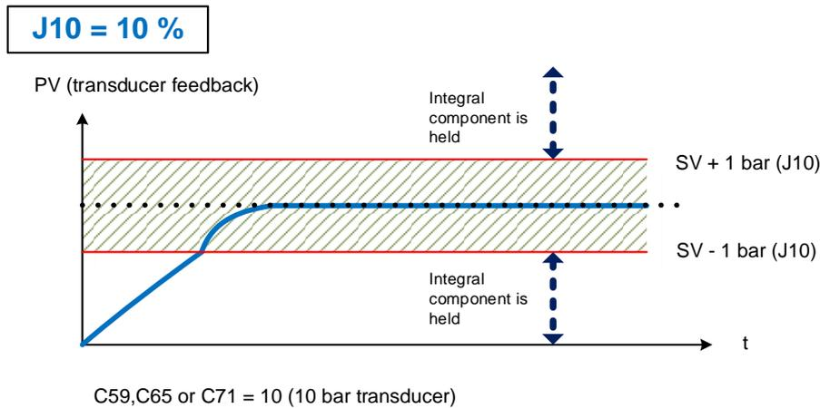
Figure 5.4: PID behaviour when function J114 is used.
