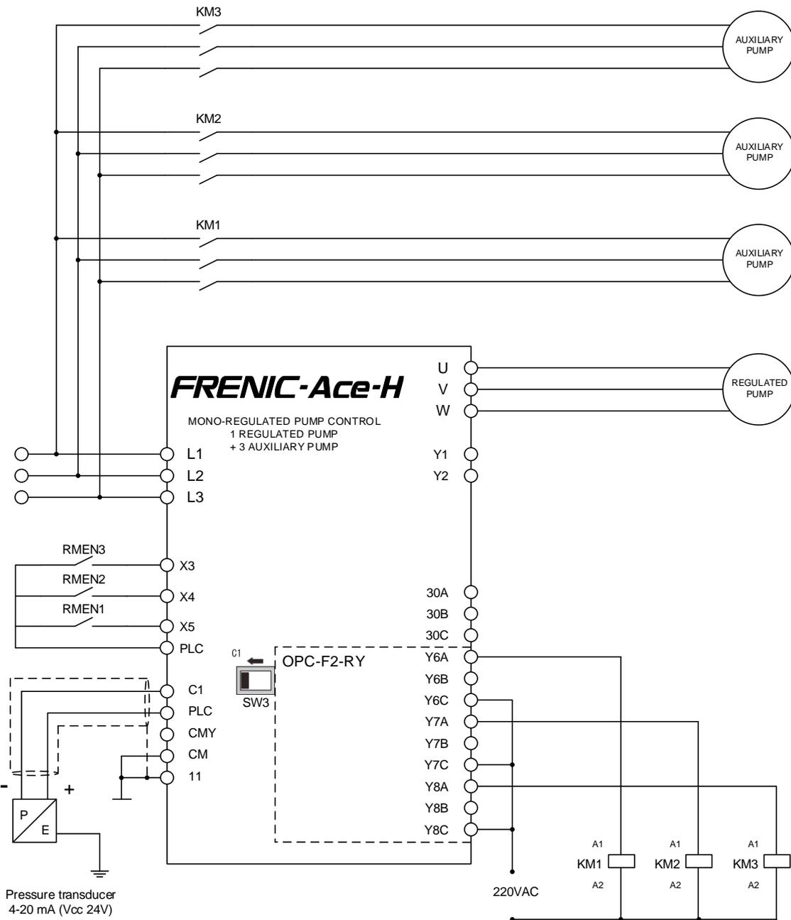
Figure 2.3: Schematic of a mono-regulated pump control with 1 regulated pump + 3 auxiliary pumps with relay option card.
