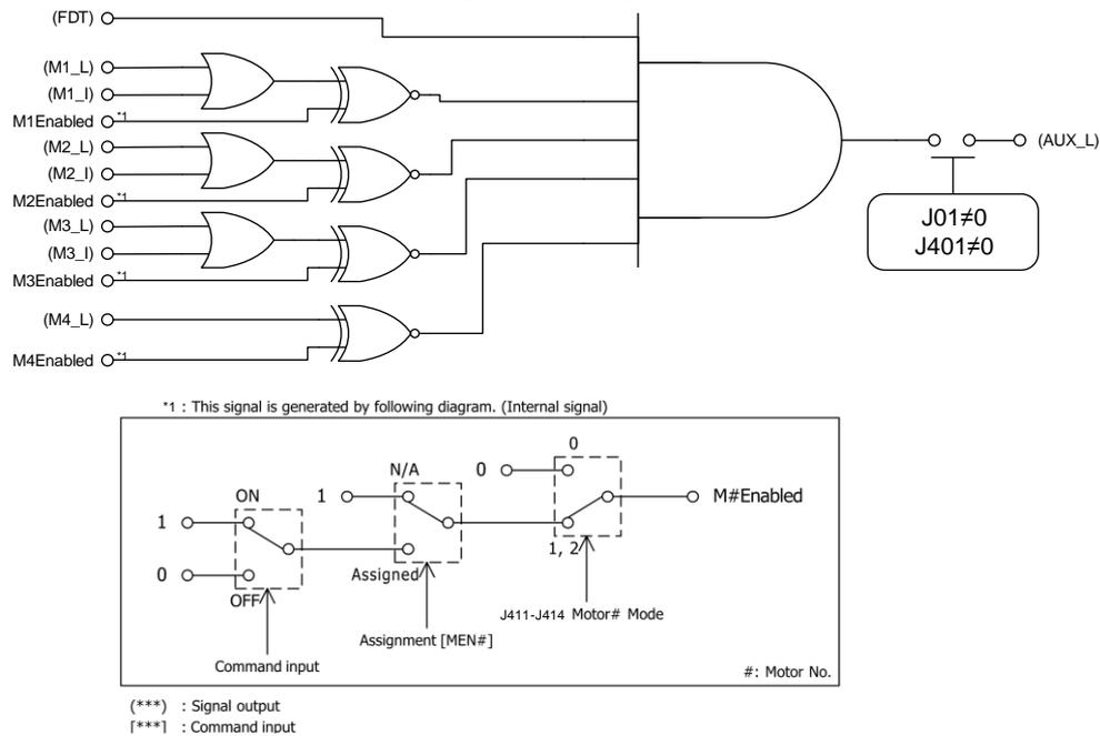
Figure 3.3: Additional pump function logic block diagram
