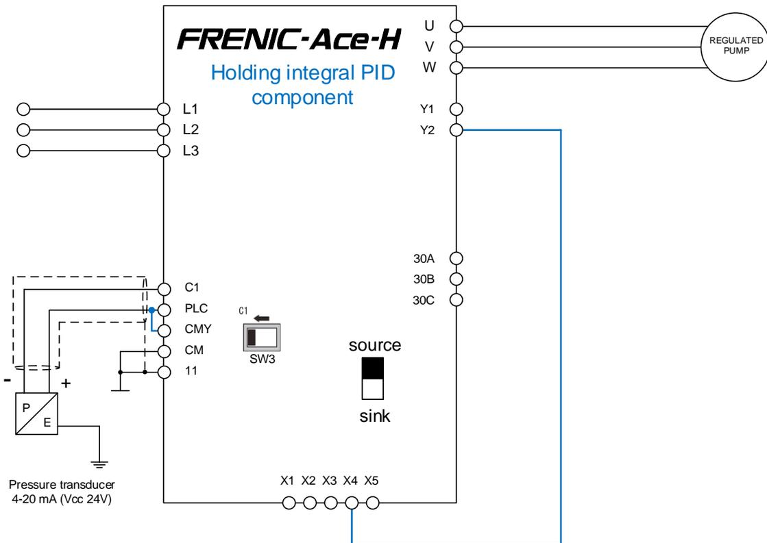
Figure 5.3: Pump control schematic for holding PID Integral component when pump is in sleep mode
