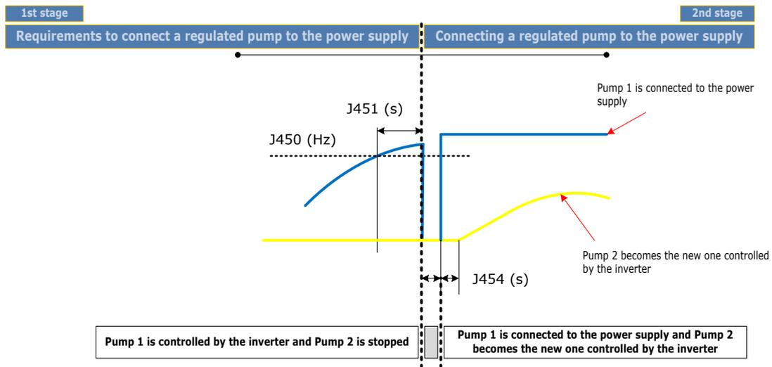
Figure 4.5: Connection of a regulated pump to the commercial power supply.
