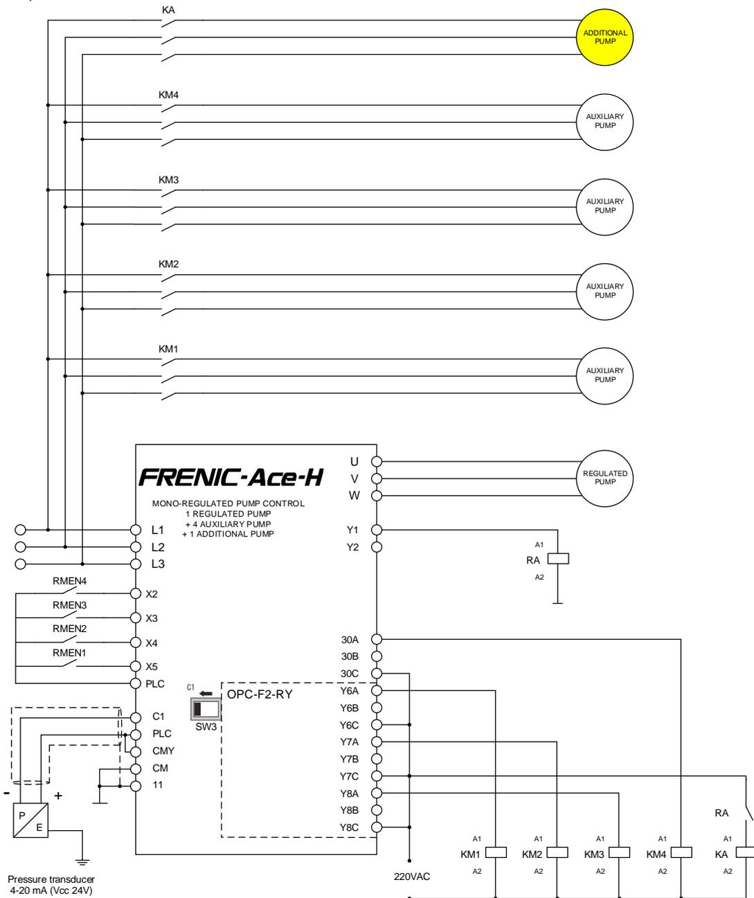
Figure 3.1: Schematic for a mono-regulated pump control with 1 regulated pump + 4 auxiliary pumps + 1 additional pump
