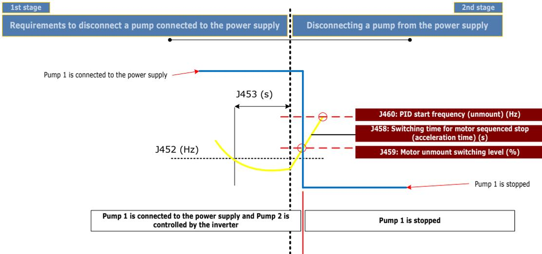
Figure 4.6: Increase of the pump's speed to disconnect the pump from the main supply
