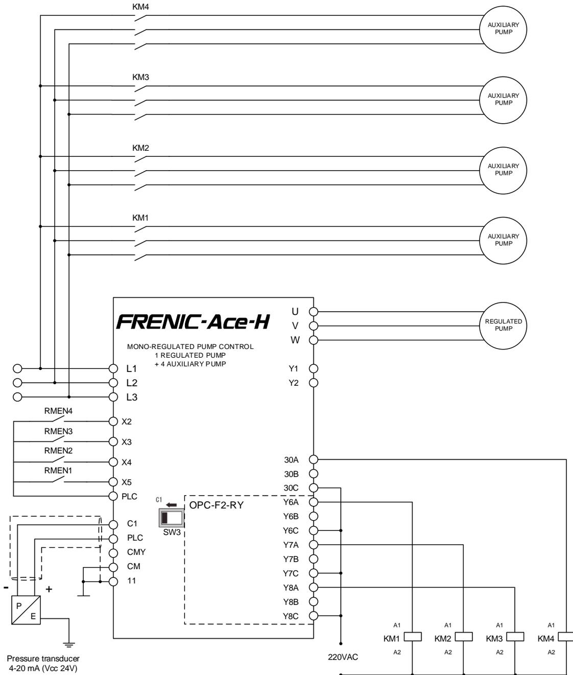
Figure 2.4: Schematic of a mono-regulated pump control with 1 regulated pump + 4 auxiliary pumps with external relays.
