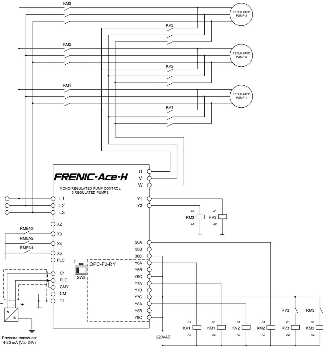
Figure 4.2: Schematics of multi-regulated pump control with 3 regulated pumps (Using OPC-F2-RY)
