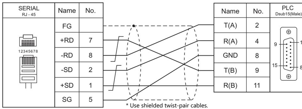
**Wiring diagram 3 - M4**
