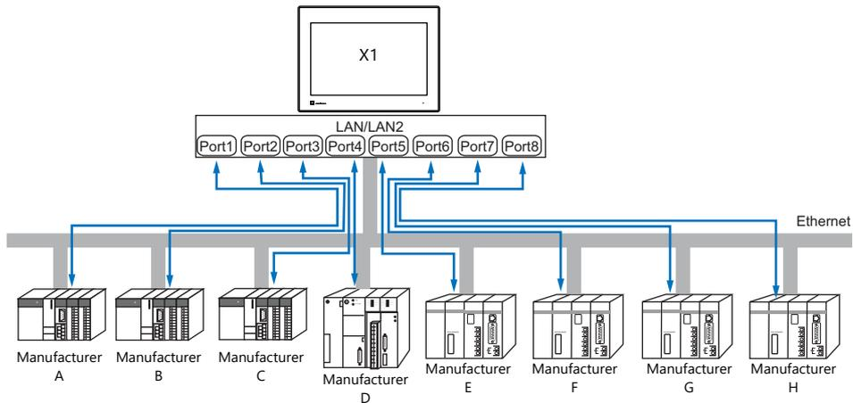
When there are two or more PLCs of the same model, the X1 series can carry out 1 : n communication via one port.
