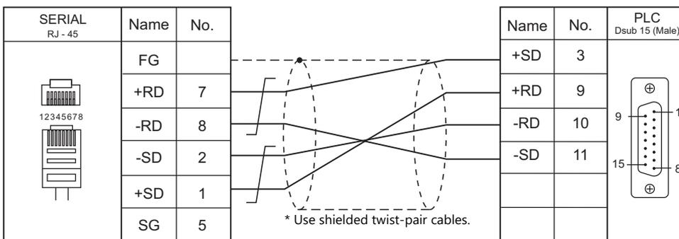
**Wiring diagram 5 - M4**
