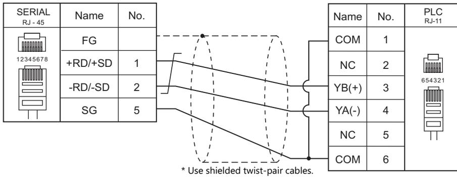
**Wiring diagram 3 - M4**
