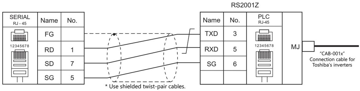
Wiring diagram 2 - M2
