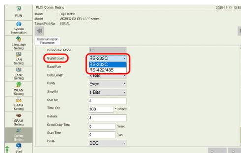
5. Press the [Apply] switch to confirm the setting.
