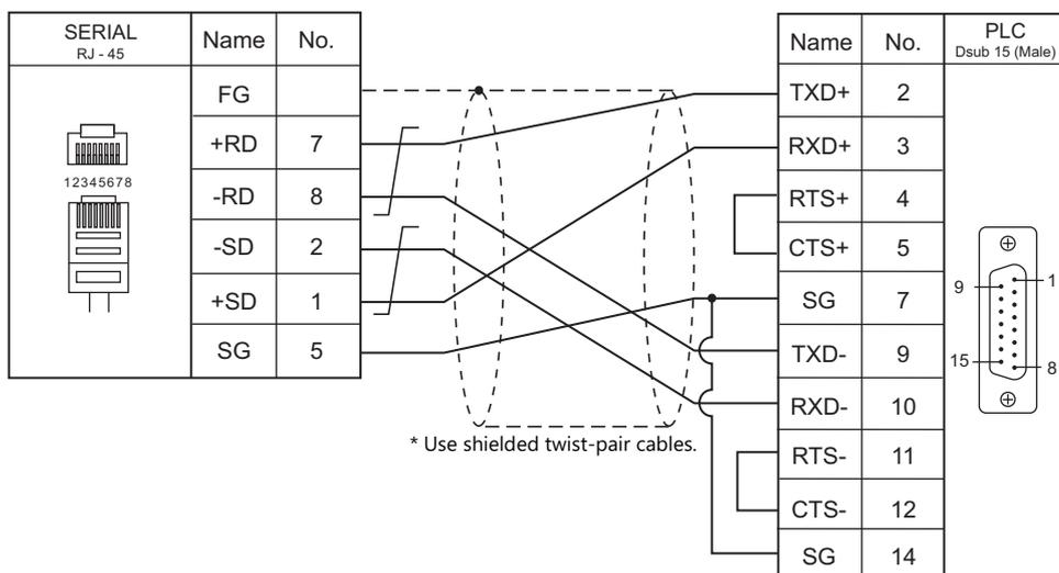
**Wiring diagram 3 - M4**
