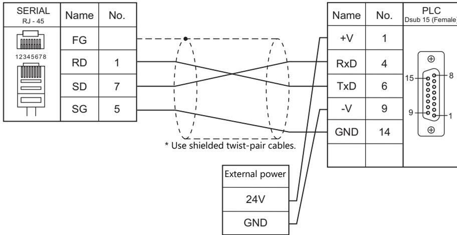
Wiring diagram 2 - M2
