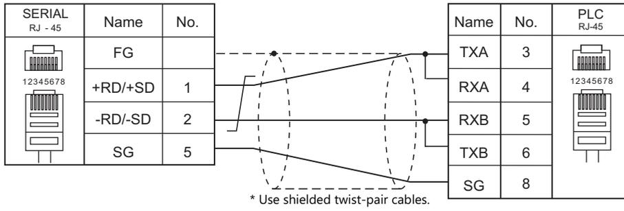
**Wiring diagram 3 - M4**
