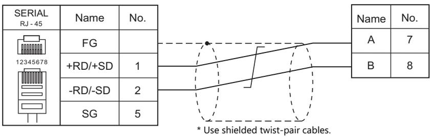
**Wiring diagram 7 - M4**
