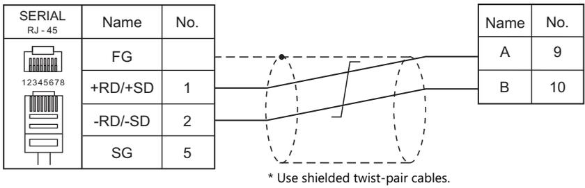
**Wiring diagram 6 - M4**
