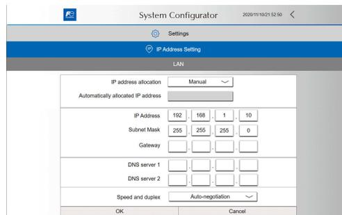
11. The IP address setting screen is displayed. Press [←].
