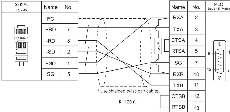
**Wiring diagram 3 - M4**
