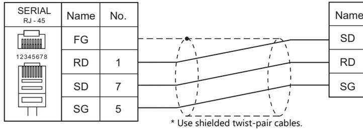
Wiring diagram 2 - M2
