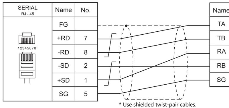
**Wiring diagram 3 - M4**
