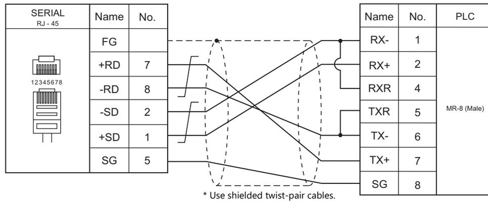
**Wiring diagram 10 - M4**
