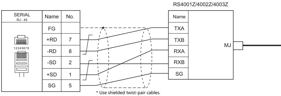
**Wiring diagram 5 - M4**
