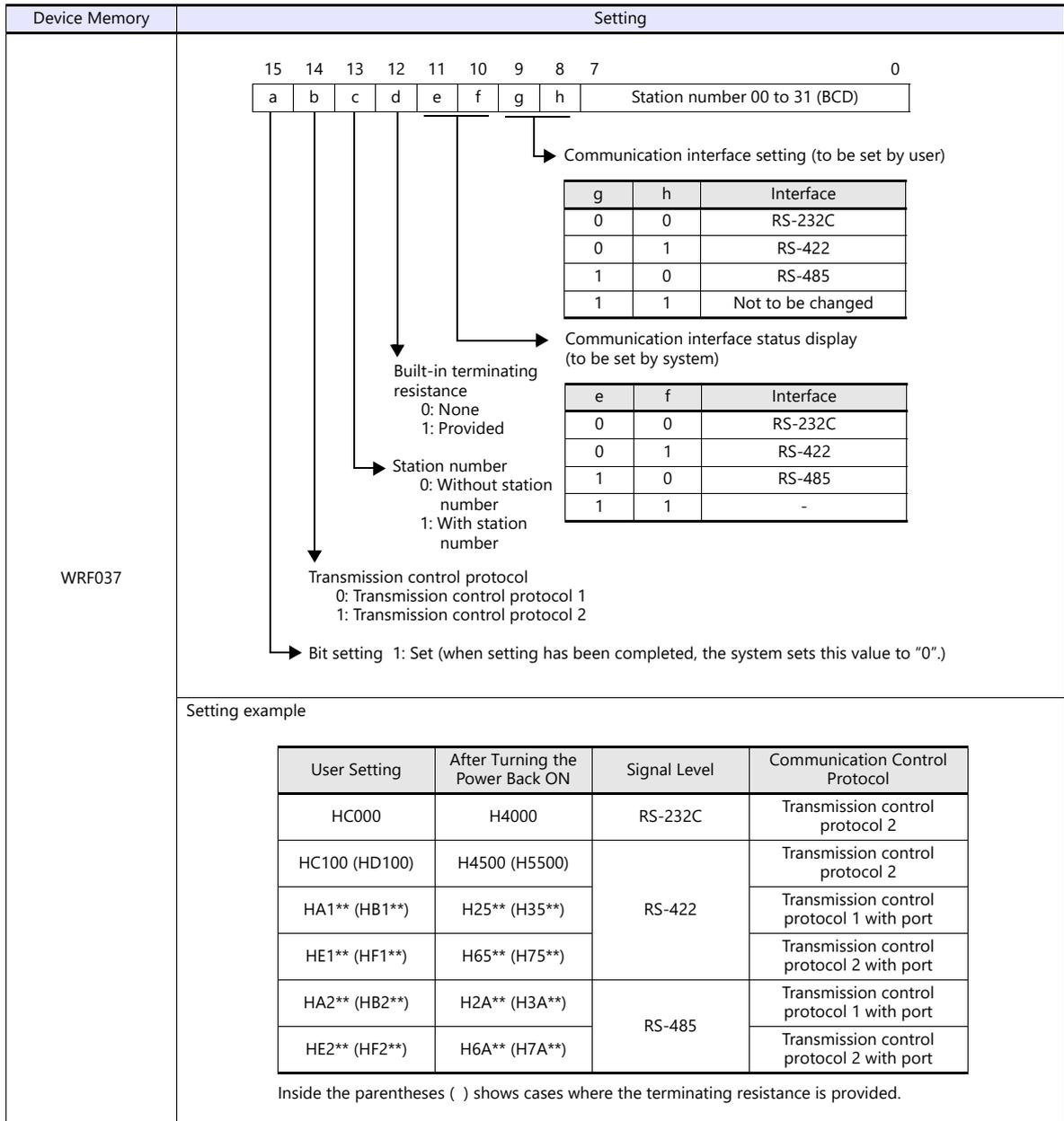
\* If the setting is undefined upon power-up, the default setting (transmission control protocol 1, without port, RS-232C) is applied. Configure the settings as required.
