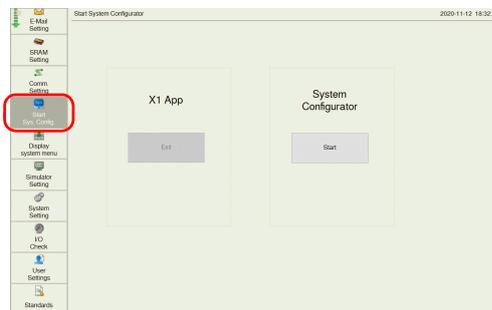
4. Press the [Start] switch. System Configurator starts.
