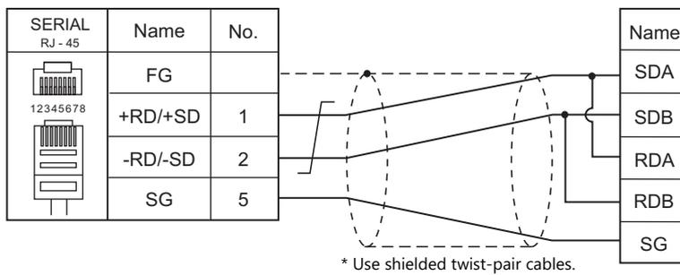
**Wiring diagram 3 - M4**
