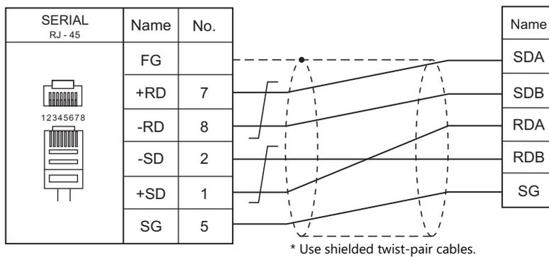
**Wiring diagram 3 - M4**
