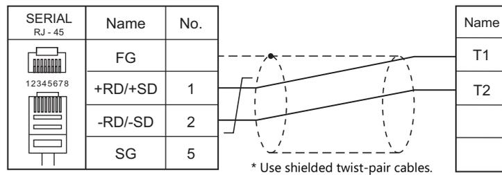
**Wiring diagram 14 - M4**
