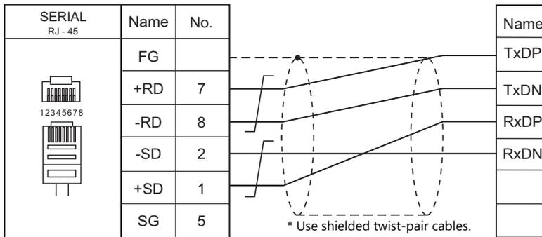
**Wiring diagram 7 - M4**
