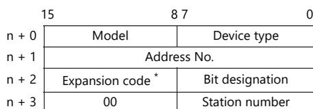
\* In the expansion code, set which word, higher or lower, is to be read when a double-word address is specified.
