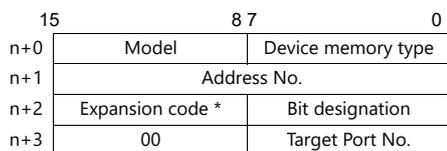
\* In the expansion code, set which word, higher or lower, is to be read when a double-word address is specified.
