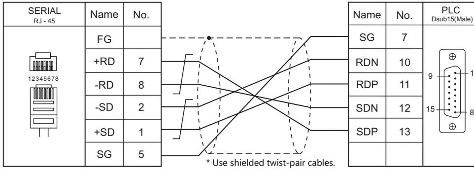
**Wiring diagram 10 - M4**
