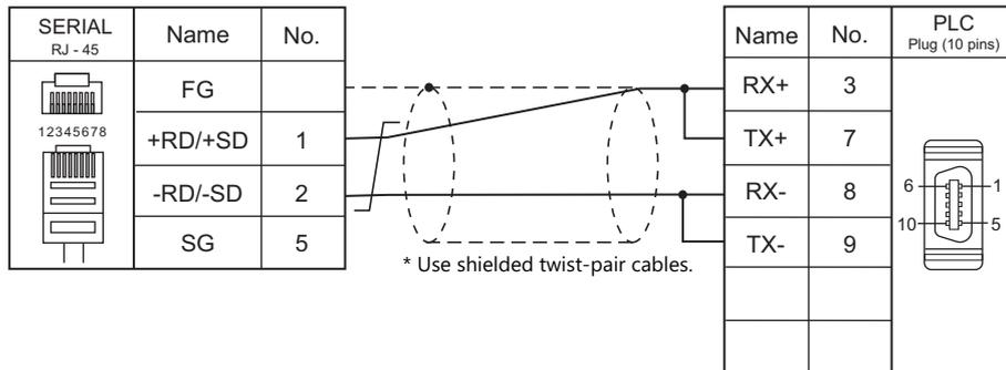
**Wiring diagram 10 - M4**
