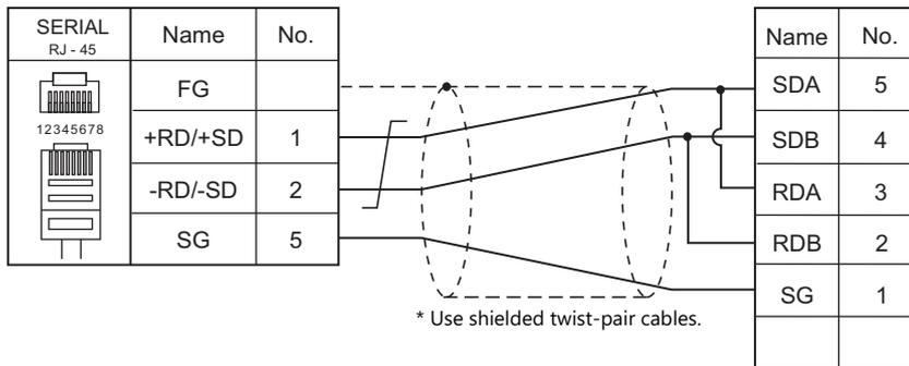
**Wiring diagram 5 - M4**
