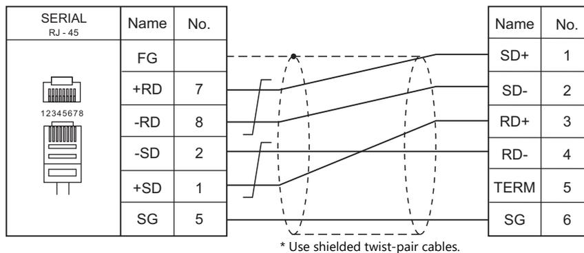
**Wiring diagram 9 - M4**
