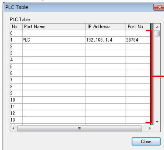
Set the IP address, port number and whether or not to use the KeepAlive function of the PLC.
