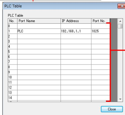
Set the IP address, port number 1025 and whether or not to use the KeepAlive function of the PLC.
