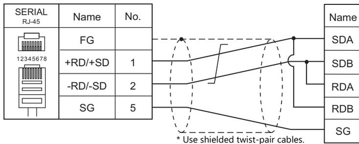
**Wiring diagram 12 - M4**
