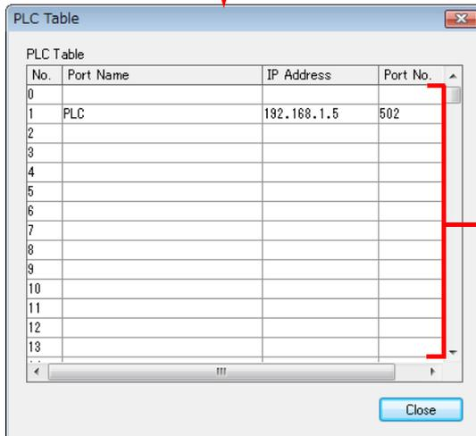
Set the IP address, port number and whether or not to use the KeepAlive function for the PLC.
