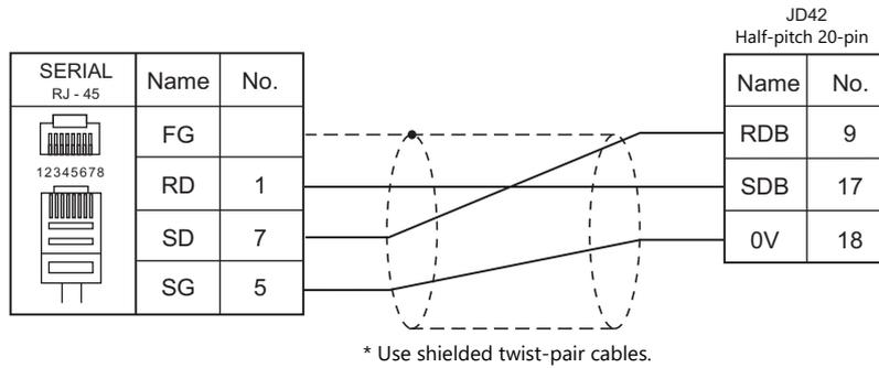
Wiring diagram 2 - M2
