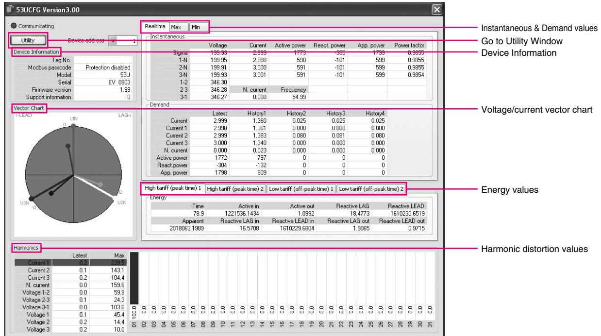
Once the PC has started communicating with the connected device, display values are updated in approx. 0.5 second intervals.
