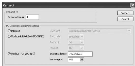
Specify the IP address (Station address) and Service port (Standard Modbus TCP port number is '502').
