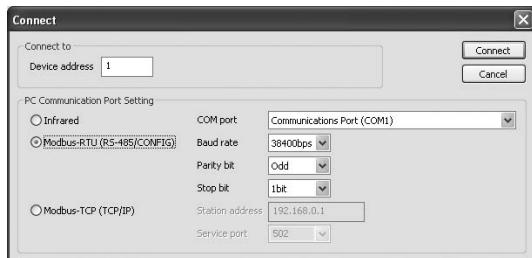
Specify the relevant device address. Specify also the COM port and Modbus communication parameters depending upon the network configuration and the device's communication parameters.
