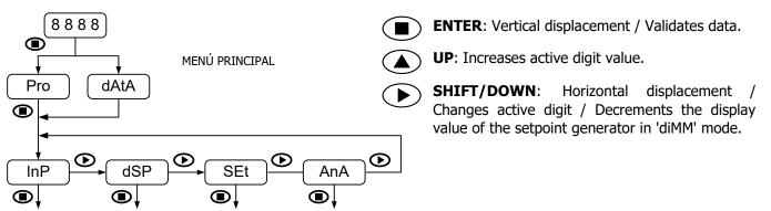
Once inside each menu, all configuration parameters are sequentially shown and they can then be introduced or edited by pressing **ENTER** key. Numeric values must be entered digit by digit, first selecting digit and then changing its value. When the display reach desired value, a new **ENTER** key pressing validates data and routine goes forward to next configuration step.
