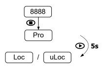
To enable / disable the adjustment of the analog output when the setpoint generator is activated, press the '**ENTER**' key and while the indication "**Pro**" is displayed, press the '**SHIFT**' / '**DOWN**' key for at least 5 seconds.
