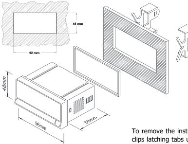
To install the instrument, prepare a 92x45mm panel cut-out and slide the unit inwards making sure of placing the sealing gasket between the front side panel and the frontal bezel.
