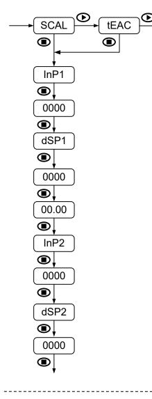
When programmed input type is process, for both display scaling "**SCAL**" and "**tEAC**" methods, parameters to be sequentially introduced are identical.
