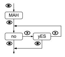
When the lock is activated (by selecting "**yES**") it is not possible to display the maximum and minimum values by means of the '**SHIFT**' key, although internally the instrument continues detecting and memorizing the extreme values reached by the input signal.
