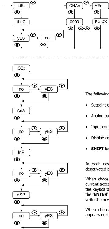
When choosing "LISt" the indication "tLoC" appears for a moment. Choosing "yES" again activates the total block and jumps directly to the MAX / MIN function lock setting, then returns to RUN mode. When the device is completely blocked, all the configuration can be accessed, although it will not be possible to enter and / or modify data. When you enter the main menu, "dAtA" will appear instead of "Pro".
