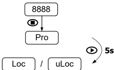
To enable / disable the adjustment of the analog output when the setpoint generator is activated, press the '**ENTER**' key and while the indication "**Pro**" is displayed, press the '**SHIFT**' / '**DOWN**' key for at least 5 seconds.
