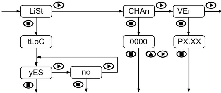
When choosing "LiSt" the indication "tLoC" appears for a moment. Choosing "yES" again activates the total block and jumps directly to the **MAX / MIN** function lock setting, then returns to **RUN** mode. When the device is **completely blocked**, all the configuration can be accessed, **although it will not be possible to enter and / or modify data**. When you enter the main menu, "dAtA" will appear instead of "Pro".
