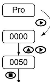
To adjust the value of the setpoint generator in programmed mode 'ProG', from the 'run' mode press the **ENTER** key and while the indication "Pro" is shown, press the **SHIFT** / **DOWN** key.
