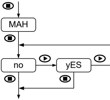
When the lock is activated (by selecting "**yES**") it is not possible to display the maximum and minimum values by means of the '**SHIFT**' key, although internally the instrument continues detecting and memorizing the extreme values reached by the input signal.
