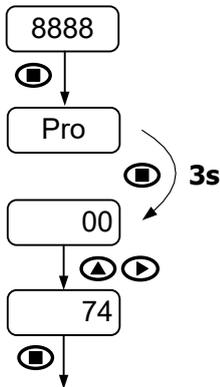
To access this menu from **RUN** mode, press **ENTER** key and while display shows "**Pro**" press again **ENTER** for at least 3 seconds.
