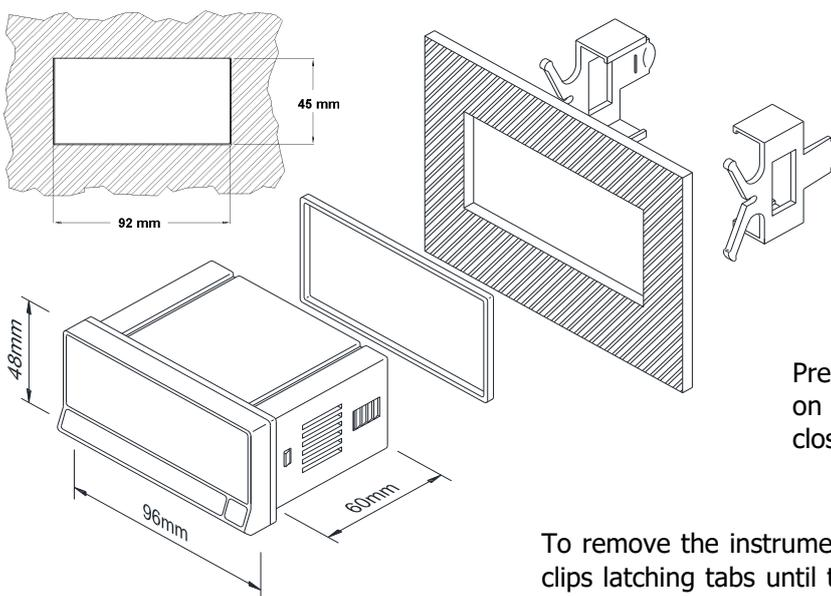
To install the instrument, prepare a 92x45mm panel cut-out and slide the unit inwards making sure of placing the sealing gasket between the front side panel and the frontal bezel.
