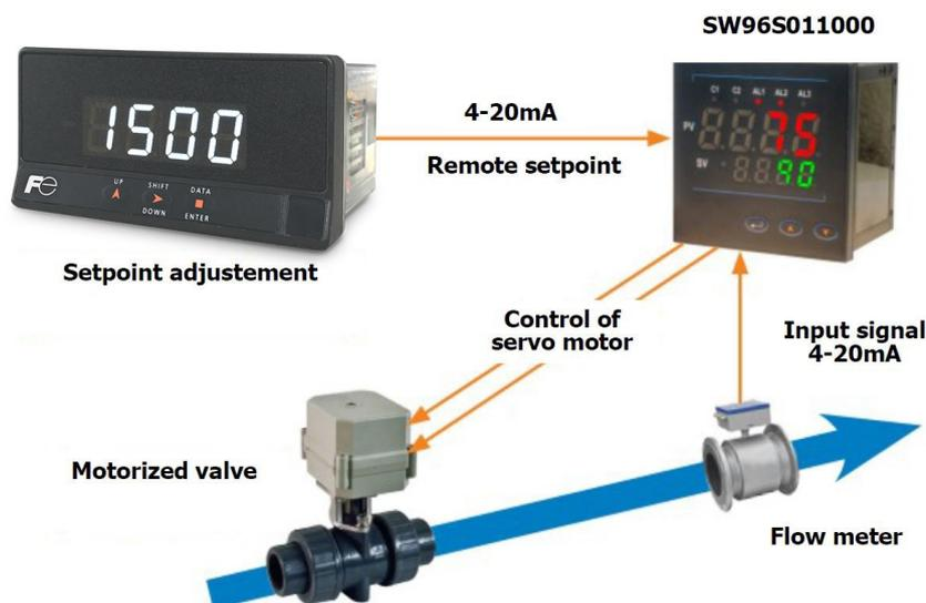
Application example. Sending remote setpoint to a device that regulates a motorized valve and controls its action by reading a flow meter.
