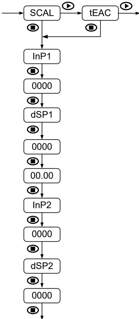
When programmed input type is process, for both display scaling "SCAL" and "tEAC" methods, parameters to be sequentially introduced are identical.
