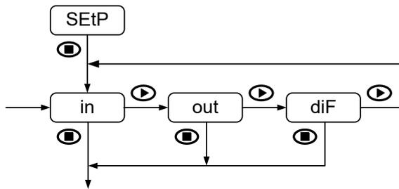
The third menu corresponds to the relay output. For more details on the operating modes, consult the section corresponding to this output later in this manual.
