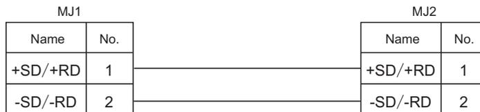
3. Press the [Self-Loop Test] switch. The test is successful if the [OK] lamp illuminates.
