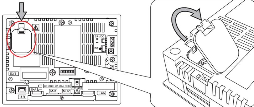
3. Insert a non-conducting precision screwdriver (flat-head screwdriver) into the gap under the battery and lift the battery out.
