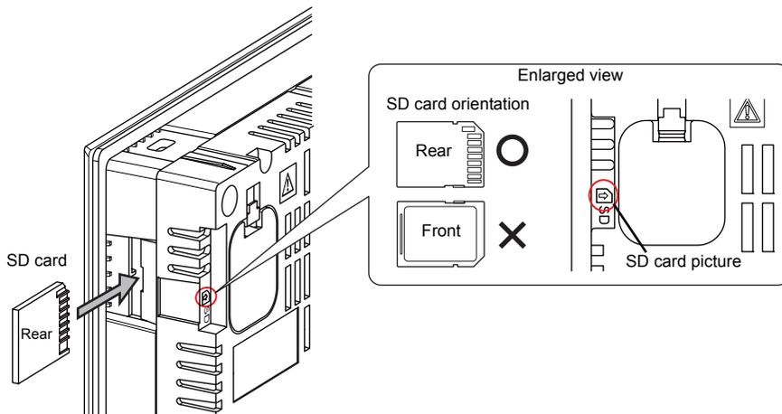
2. Push the SD card until it clicks and then the SD card will come out. Pinch the SD card with your fingers and remove it from the slot.
