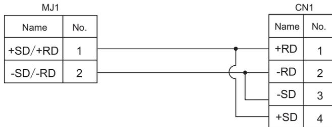
2. Press the [Self-Loop Test] switch. The test is successful if the [OK] lamp illuminates.
