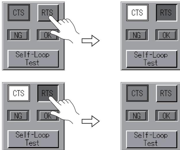
\* The loopback test is performed using [+RD] (pin 1) and [-RD] (pin 2) because the CN1 (D-sub 9-pin) connector does not have [+CTS] and [-CTS].
