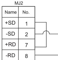
3. Press the [Self-Loop Test] switch. The test is successful if the [OK] lamp illuminates.
