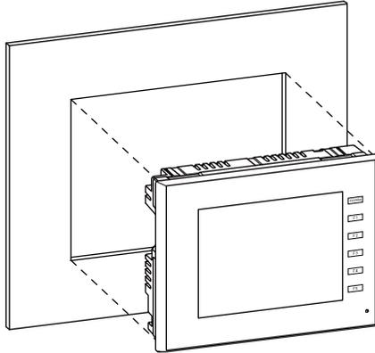
2. Insert the four fixtures provided with the TS2060 unit into the mounting holes and tighten them with the tightening screws (tightening torque: 4.43 lbf-in (0.5 N·m)).
