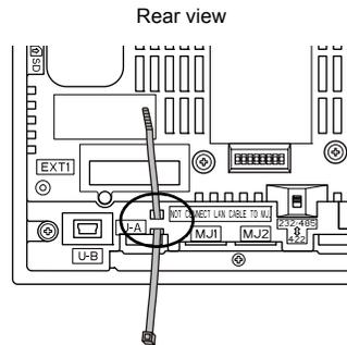
2. Inserting and securing a USB cable
