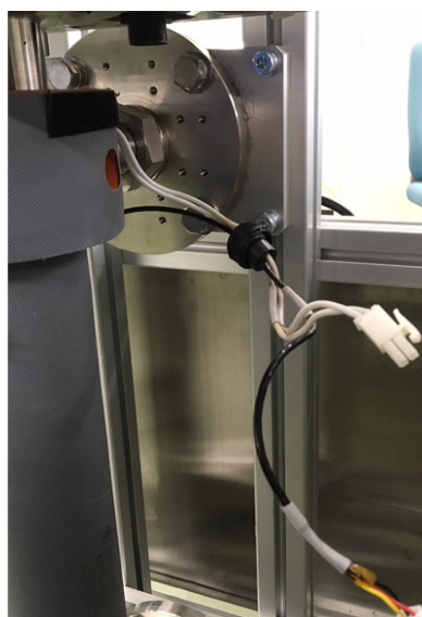
Photo 3-21 Cable ground outside the receiver unit (left). Disconnect the cable gland and pull out the heater cable (right)
