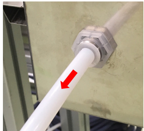
Photo 1-4 Pull the tube with a force of 5 to 15N to confirm that it does not come off.
