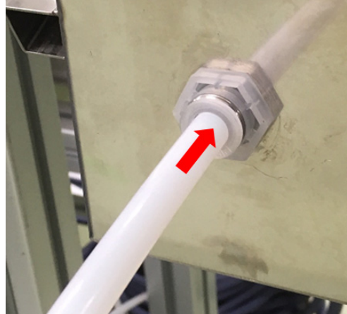
Photo 1-3 Insert the tube into the fitting and push it until it stops.
