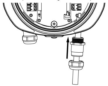
**6.** Connect the power cable to either the 24 V DC or 100 ... 240 V AC power supply terminal. Insert the wires to the terminal block and tighten the screws.
