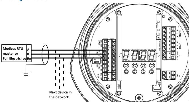
Figure 25: Modbus RTU bus on the main board
