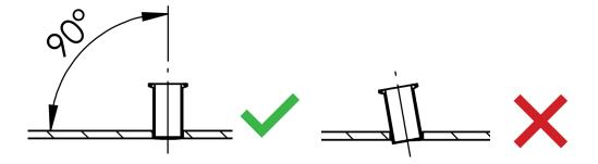
**6.** Weld the process connection to the duct or pipe. Make sure that the welding joint is airtight
