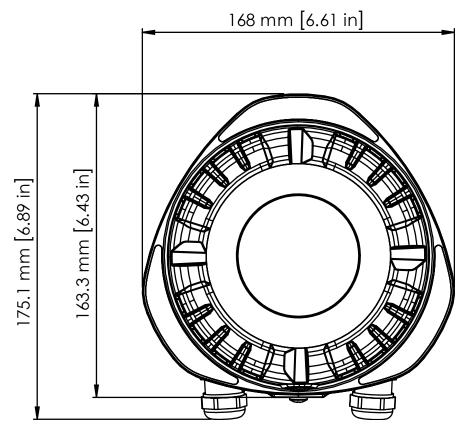
Figure 4: Front view dimensions of the enclosure
