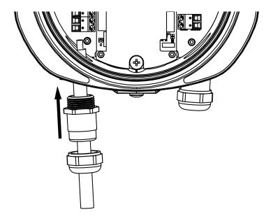
**6.** Connect the signal cable to mA output terminal block. Insert the wires to the terminal block and tighten the screws.
