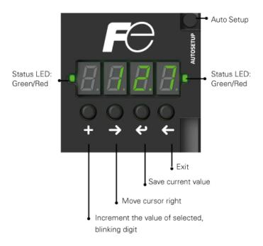
Figure 34: The main interface of the device
