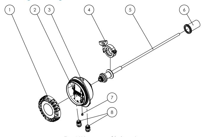
Figure 1: Main components of the dust monitor
