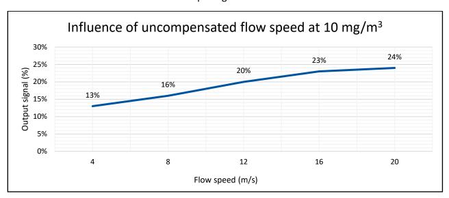
Figure 14: Influence of uncompensated flow speed on the output signal
