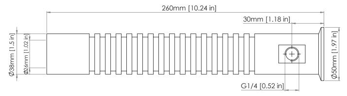
Figure 7: High-temperature process connection dimensions
