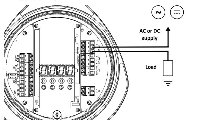
Figure 23: Relay connections on the main board
