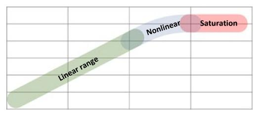
Figure 12: Uncalibrated measuring behavior
