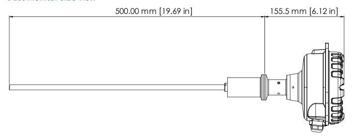
Figure 3: Side view dimensions of the enclosure and probe
