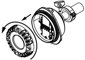
**3.** Remove the cable gland at the cable entry that is located on the right side of the device when you are facing the main board. Loosen the cable gland cap by turning it counterclockwise with a wrench.
