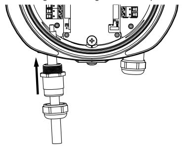
**6.** Connect the signal cable to mA input terminal block. Insert the wires to the terminal block and tighten the screws.
