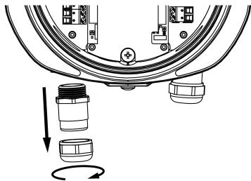
**4.** Slide the cable gland over the incoming signal cable.
