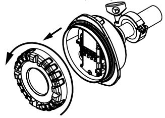
**b.** Remove the cable gland at the cable entry that is located on the right side of the device when you are facing the main board. Loosen the cable gland cap by turning it counterclockwise with a wrench.
