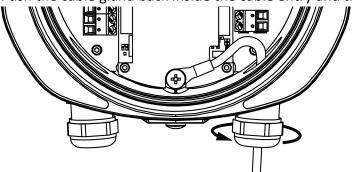
o Attach the device lid by tightening it clockwise.
