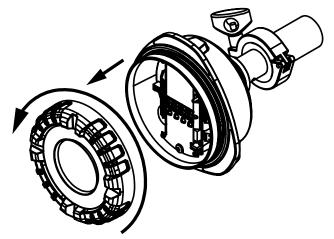
**3.** Remove the cable gland at the cable entry that is located on the left side of the device when you are facing the main board. Loosen the cable gland cap by turning it counterclockwise with a wrench.
