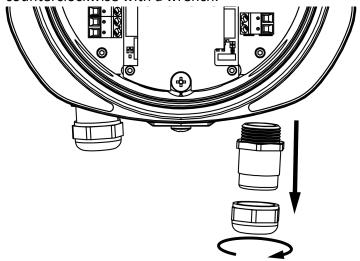
**c.** Slide the cable gland over the incoming ground wire.
