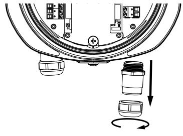
**4.** Slide the cable gland over both incoming signal cables.
