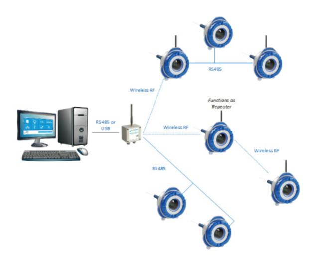
Figure 33: An example of a device network using Fuji Electric Network protocol with wired and wireless connections
