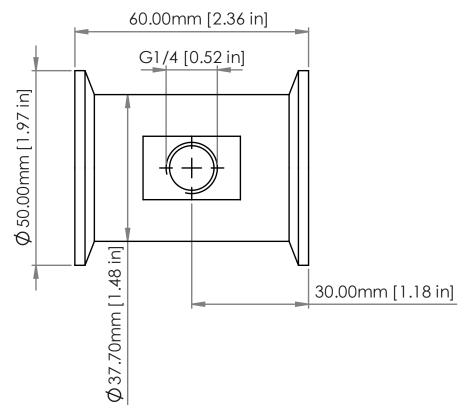
Figure 6: Air purge adapter dimensions
