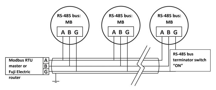
Figure 32: A device network created with RS-485 connections
