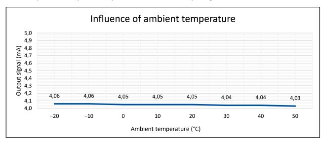
Figure 13: Influence of ambient temperature on the output signal
