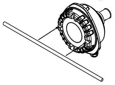
**2.** Use the rod to turn the lid counterclockwise. The slots lock the rod in place, allowing you to force the lid open.
