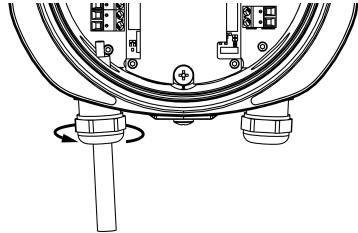
Attach the device lid by tightening it clockwise.
