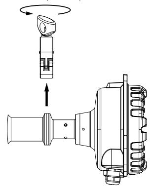
**2.** Remove the device from the process by lifting it out of the process connection. Leave the quick-clamp gasket in place on the process connection.
