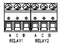
Figure 35: Relay terminals on the device main board
