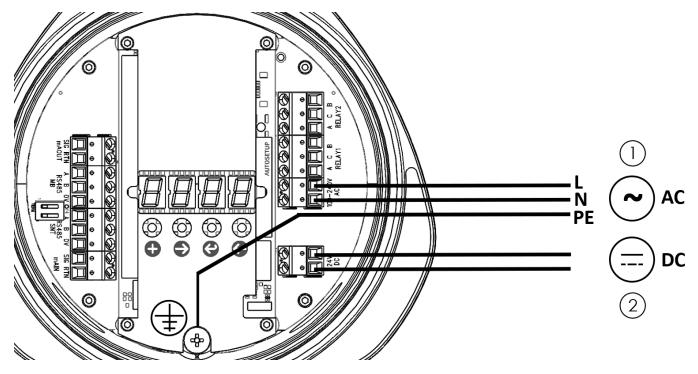
Figure 22: Power supply inputs on the main board
