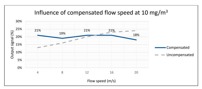
Figure 15: Influence of compensated flow speed on the output signal
