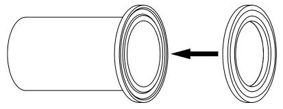
**8.** Insert the sensor probe through the process connection.
