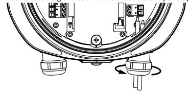
Attach the device lid by tightening it clockwise.
