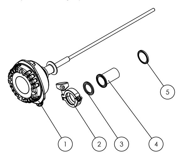
Figure 9: Components included in a standard delivery
