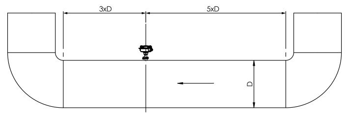
Figure 16: Recommended distance to obstacles (D = Duct diameter)
