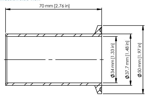
Figure 5: Process connection dimensions
