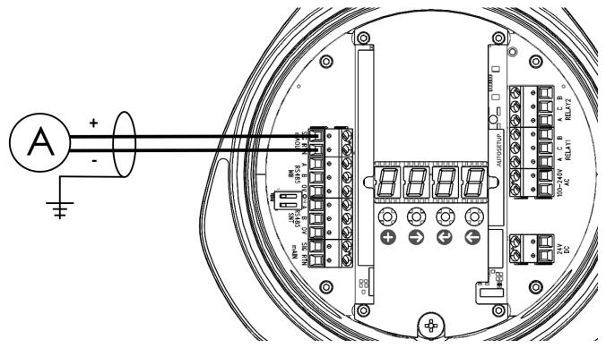
Figure 24: mA output on the main board
