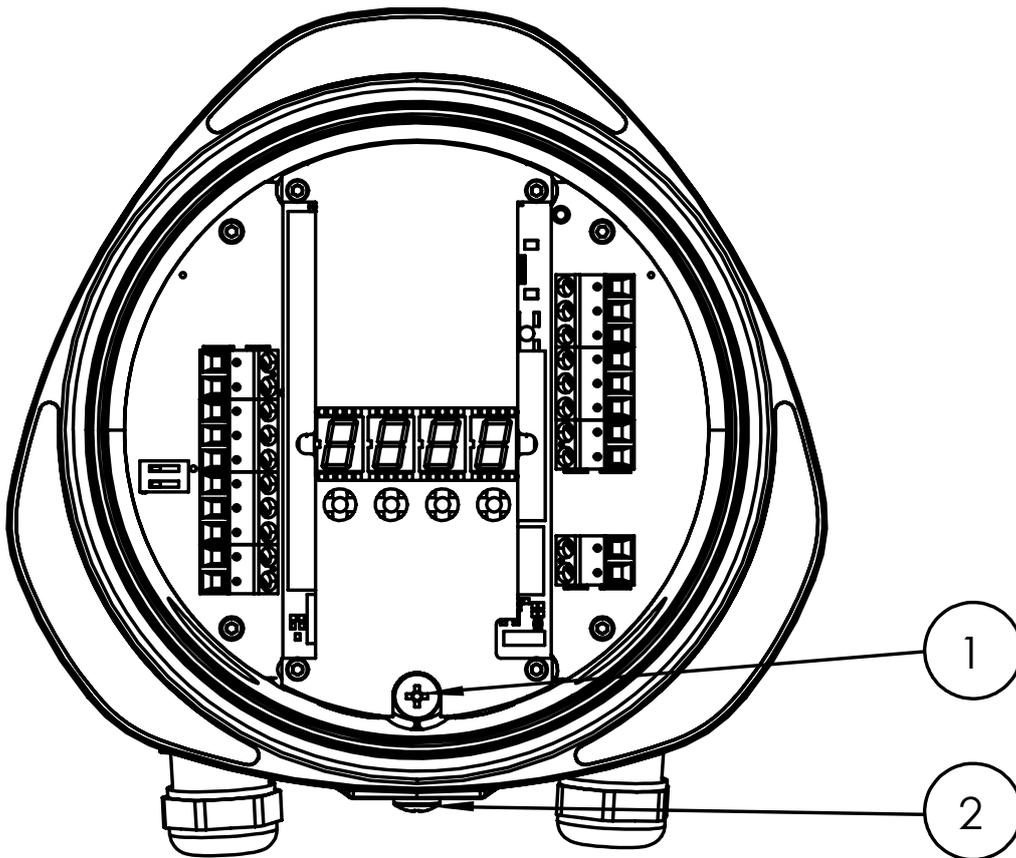
Figure 21: Position of ground connections on the enclosure
