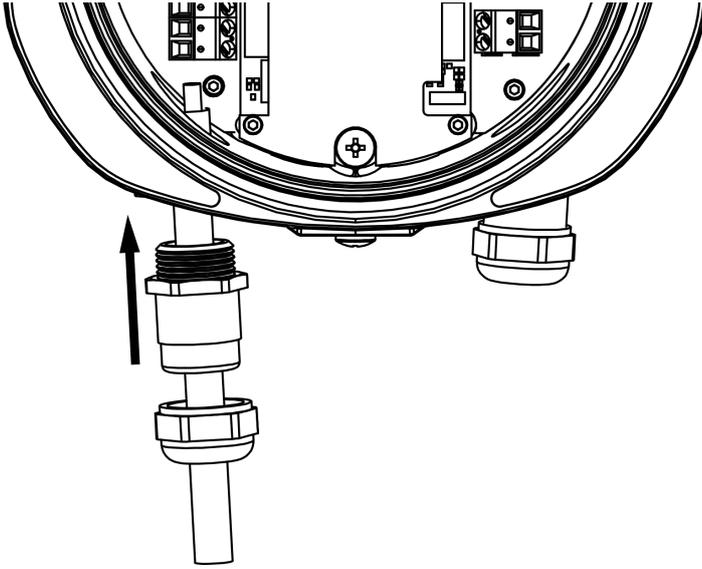
6. Connect the signal cable to mA output terminal block.
