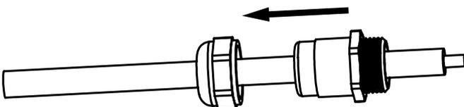
5. Insert the power cable through the cable entry.
