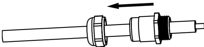
5. Insert the signal cable through the cable entry.
