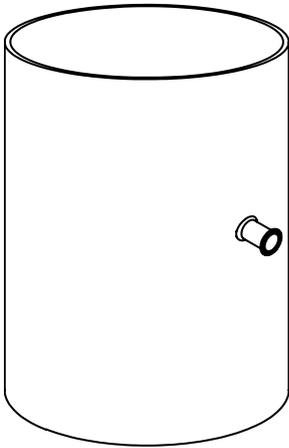
7. Fit the quick-clamp gasket on the sensor end of the process connection.
