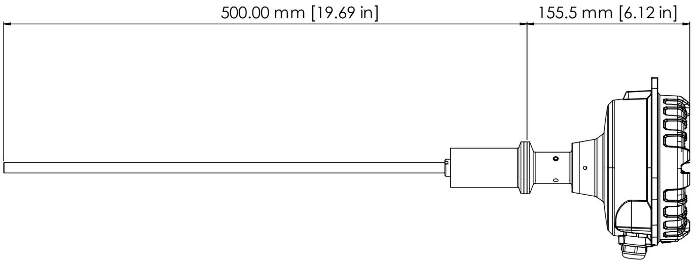
Figure 3: Side view dimensions of the enclosure and probe
