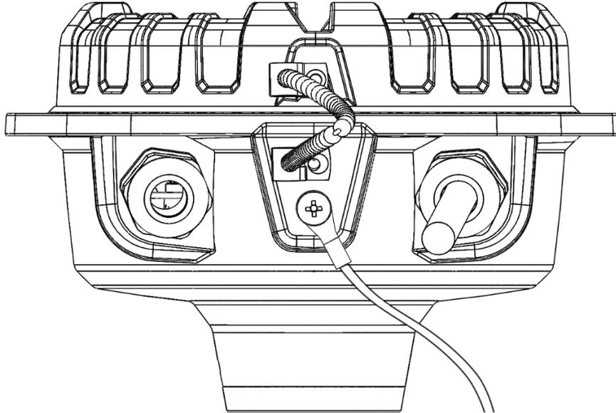
4. Connect the other end of the ground wire to a location with the same ground potential as the ductwork that the device is installed on.
