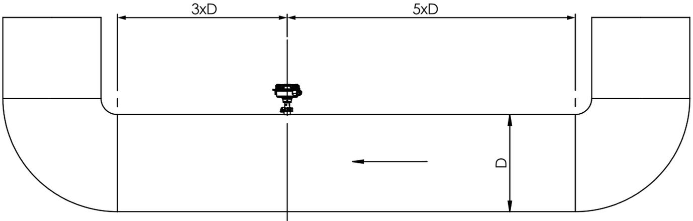
Figure 16: Recommended distance to obstacles (D = Duct diameter)
