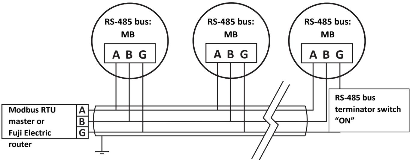
Figure 32: A device network created with RS-485 connections
