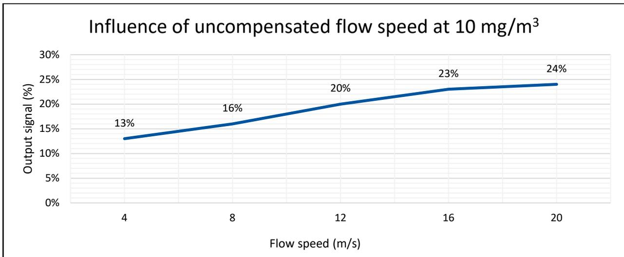
Figure 14: Influence of uncompensated flow speed on the output signal
