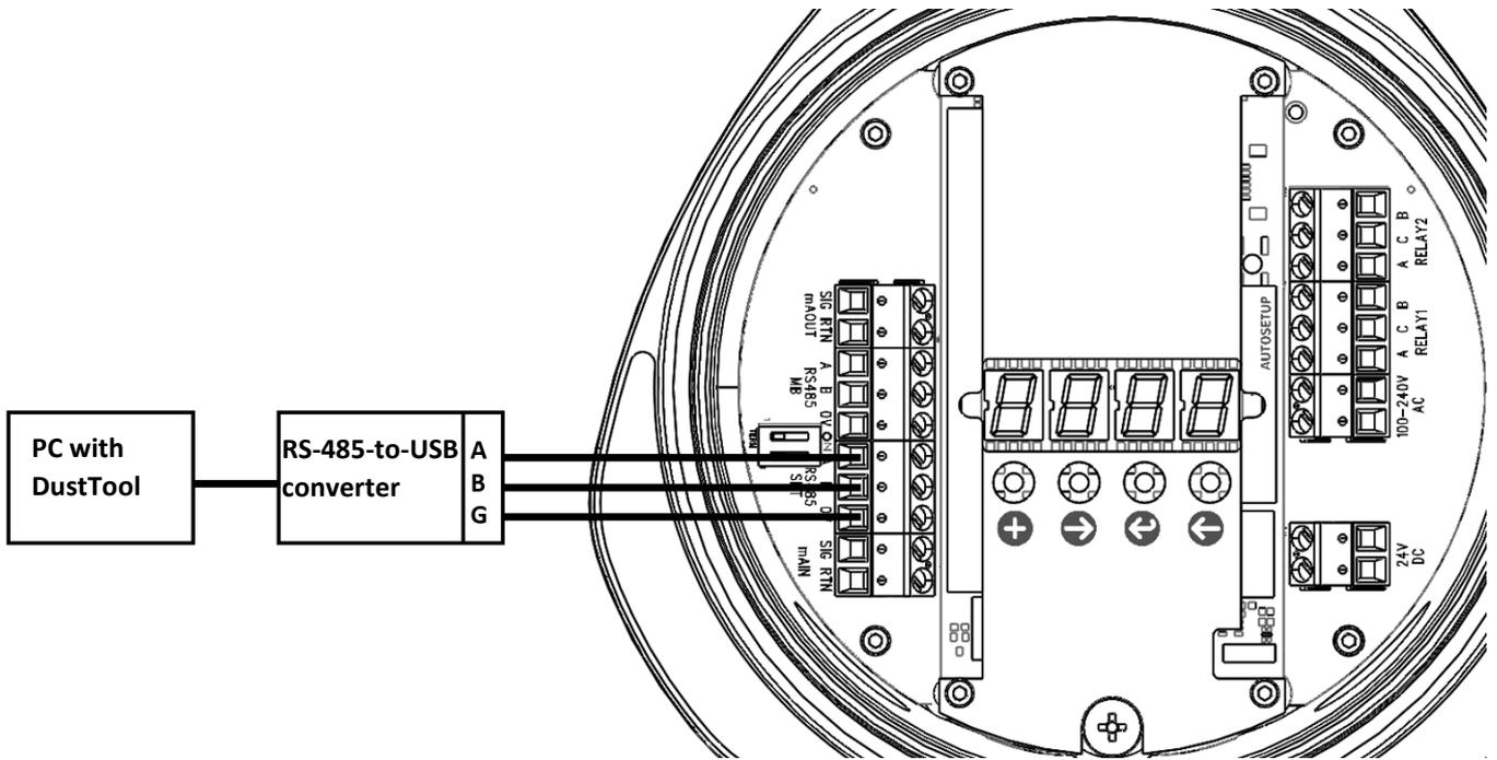
Figure 26: Fuji Electric Network bus on the main board
