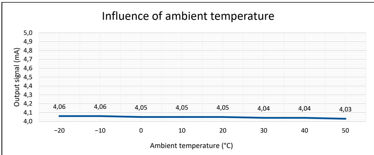
Figure 13: Influence of ambient temperature on the output signal
