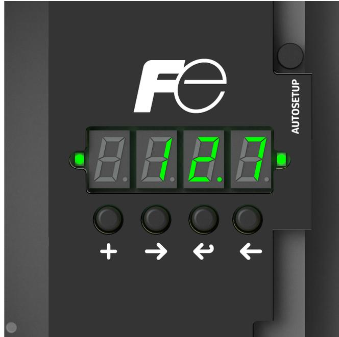
Figure 30: Main interface of the device with K0 (+) and AUTOSETUP keys highlighted
