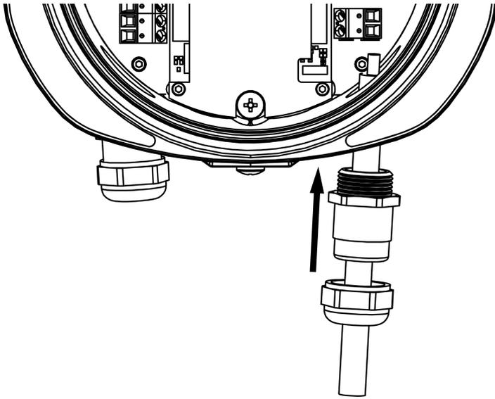
6. Connect the power cable to either the 24 V DC or 100 ... 240 V AC power supply terminal. Insert the wires to the terminal block and tighten the screws.
