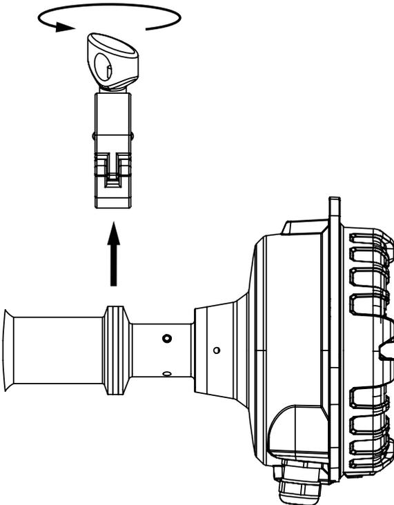
2. Remove the device from the process by lifting it out of the process connection. Leave the quick-clamp gasket in place on the process connection.
