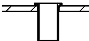
5. Make sure that the process connection is in the right position and correctly aligned. The socket must be perpendicular to the airflow inside the duct.
