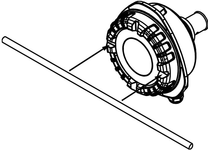
2. Use the rod to turn the lid counterclockwise. The slots lock the rod in place, allowing you to force the lid open.
