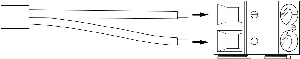
7. Connect the other end of the signal cable to the device that receives the mA output.
