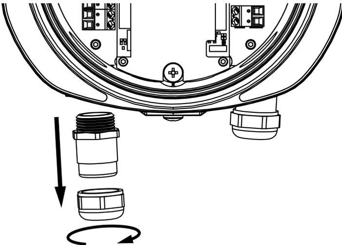
5. Slide the cable gland over the incoming signal cable.
