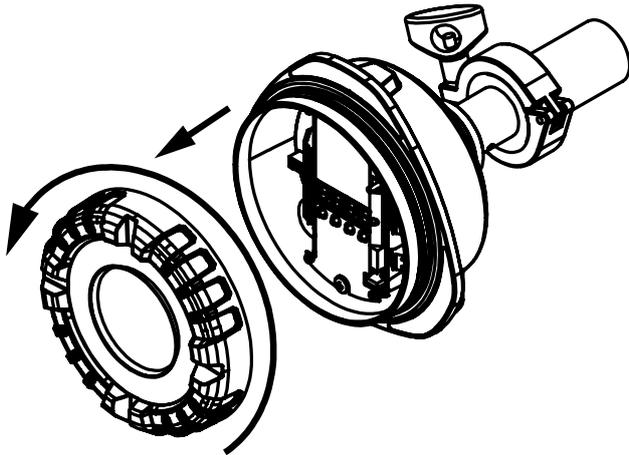
3. Remove the cable gland at the cable entry that is located on the left side of the device when you are facing the main board. Loosen the cable gland cap by turning it counterclockwise with a wrench.
