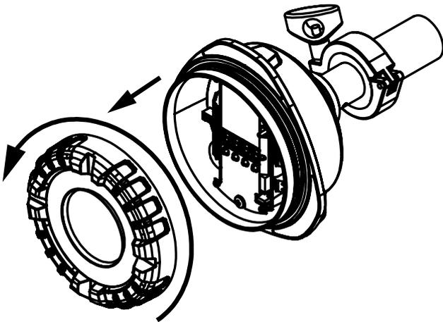
4. Remove the cable gland at the cable entry that is located on the left side of the device when you are facing the main board. Loosen the cable gland cap by turning it counterclockwise with a wrench.
