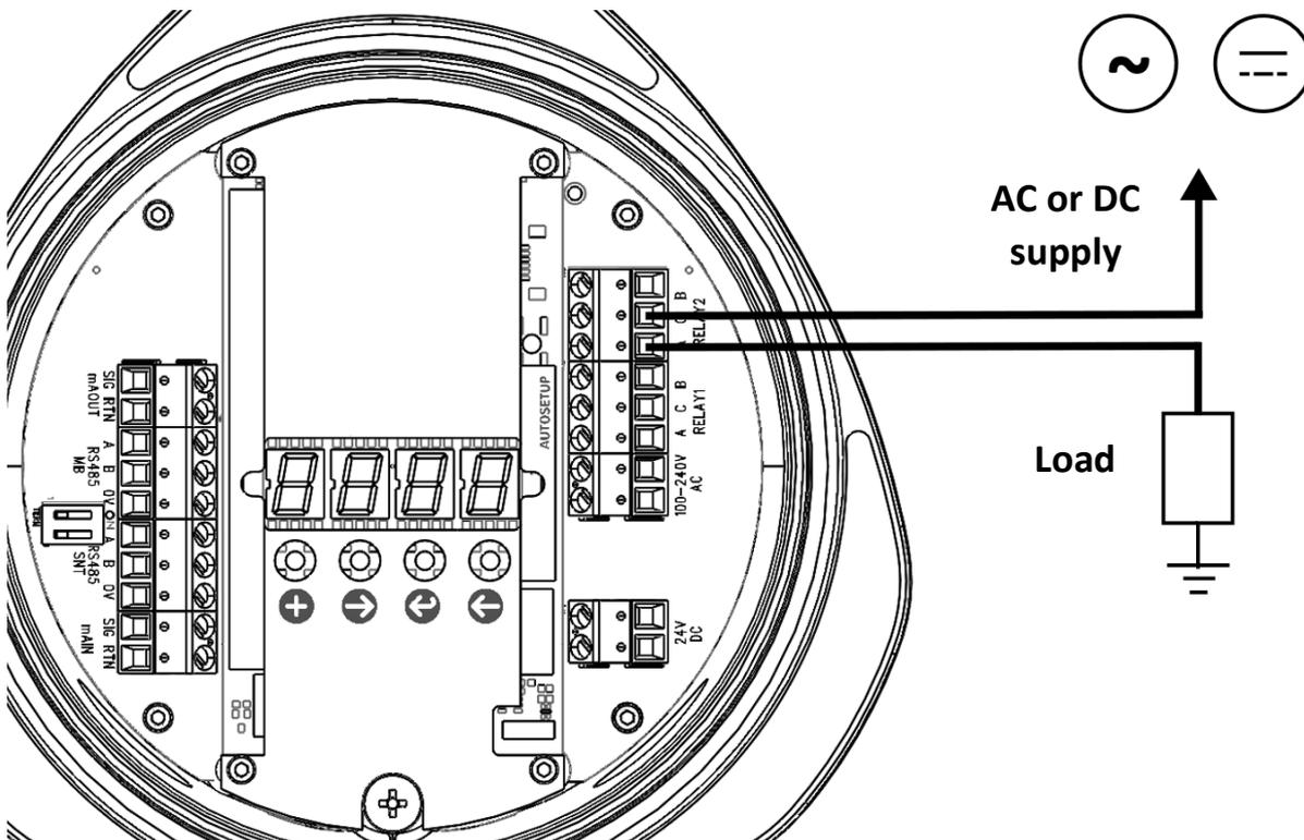
Figure 23: Relay connections on the main board
