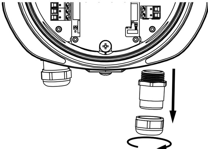
4. Slide the cable gland over both incoming signal cables.
