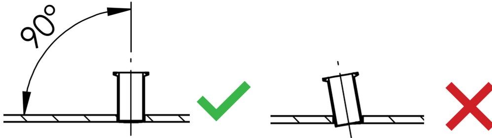
6. Weld the process connection to the duct or pipe. Make sure that the welding joint is airtight
