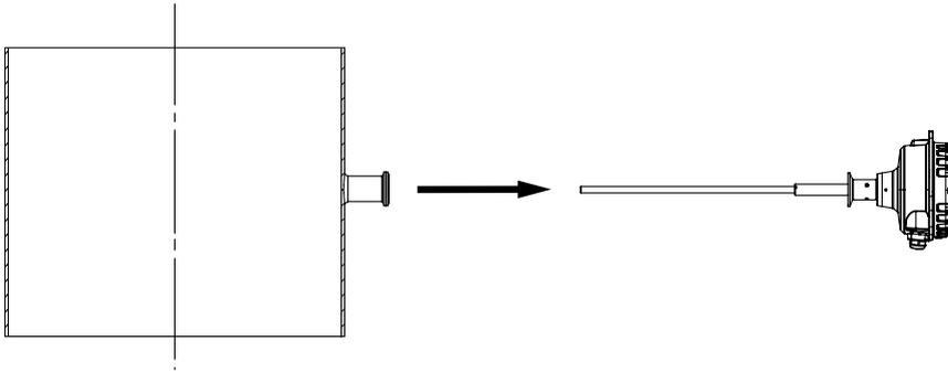
3. Fit the end cap on the process connection.
