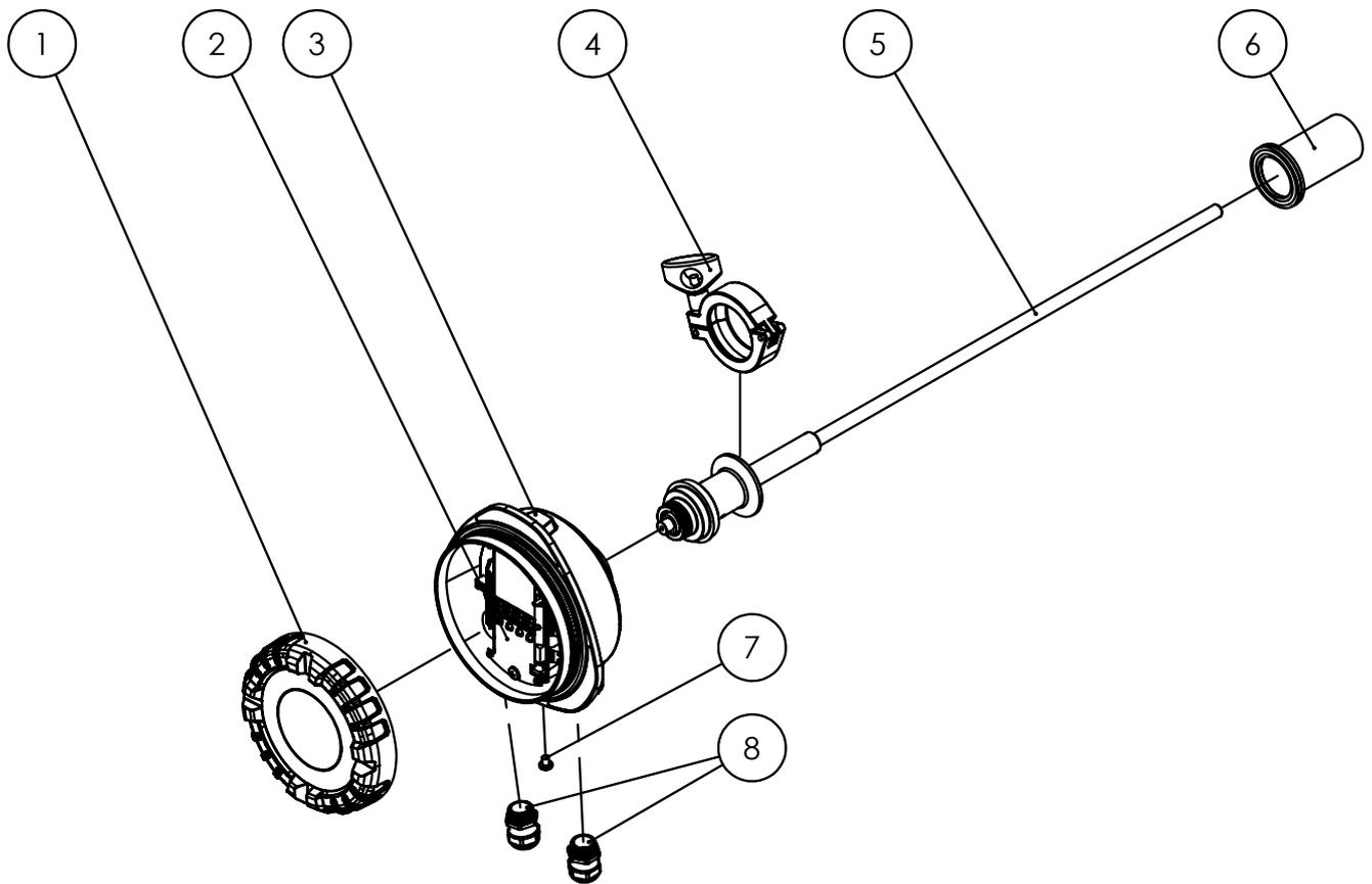
Figure 1: Main components of the dust monitor
