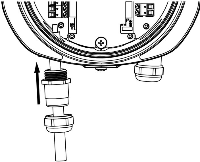
6. Connect the signal cable to mA input terminal block.
