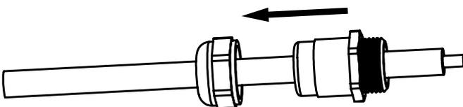
6. Insert the signal cable through the cable entry.
