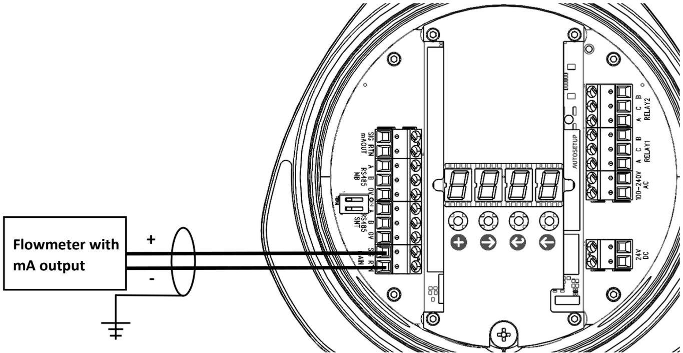
Figure 27: mA input on the main board
