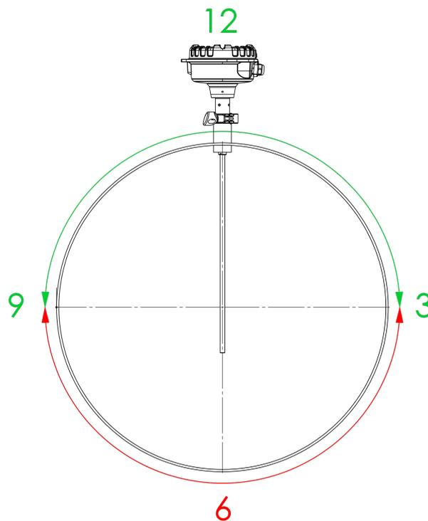
Figure 18: Approved installation positions on a round duct
