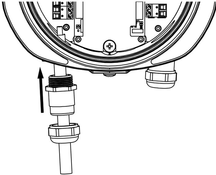
7. Connect the signal cable to the RS-485 output terminal block.
