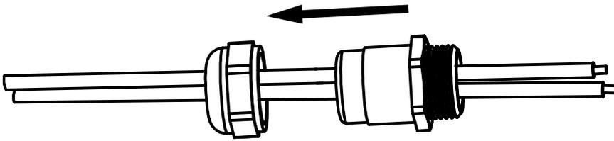
5. Insert both signal cables through the cable entry.
