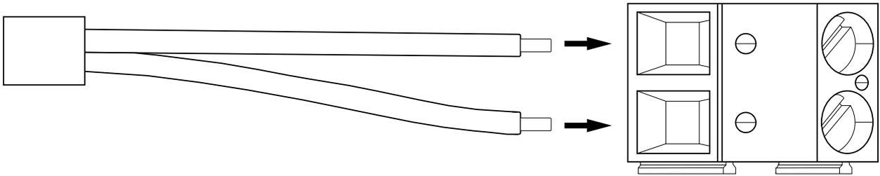
7. Connect the other end of the signal cable to the mA output of the external flowmeter.
