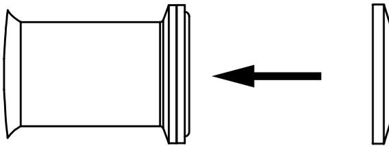
4. Secure the end cap in place with the quick-clamp connector.
