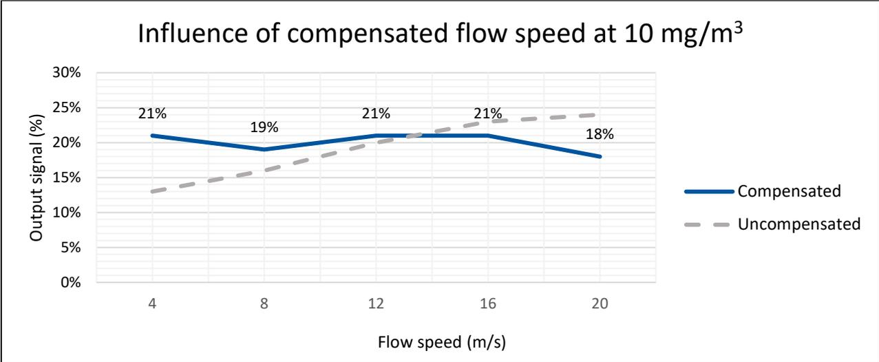
Figure 15: Influence of compensated flow speed on the output signal
