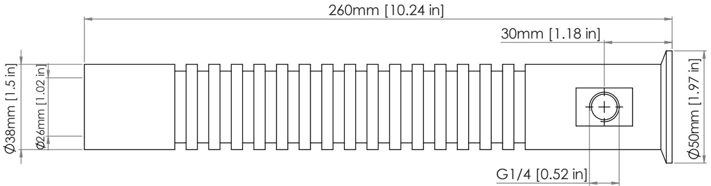
Figure 7: High-temperature process connection dimensions
