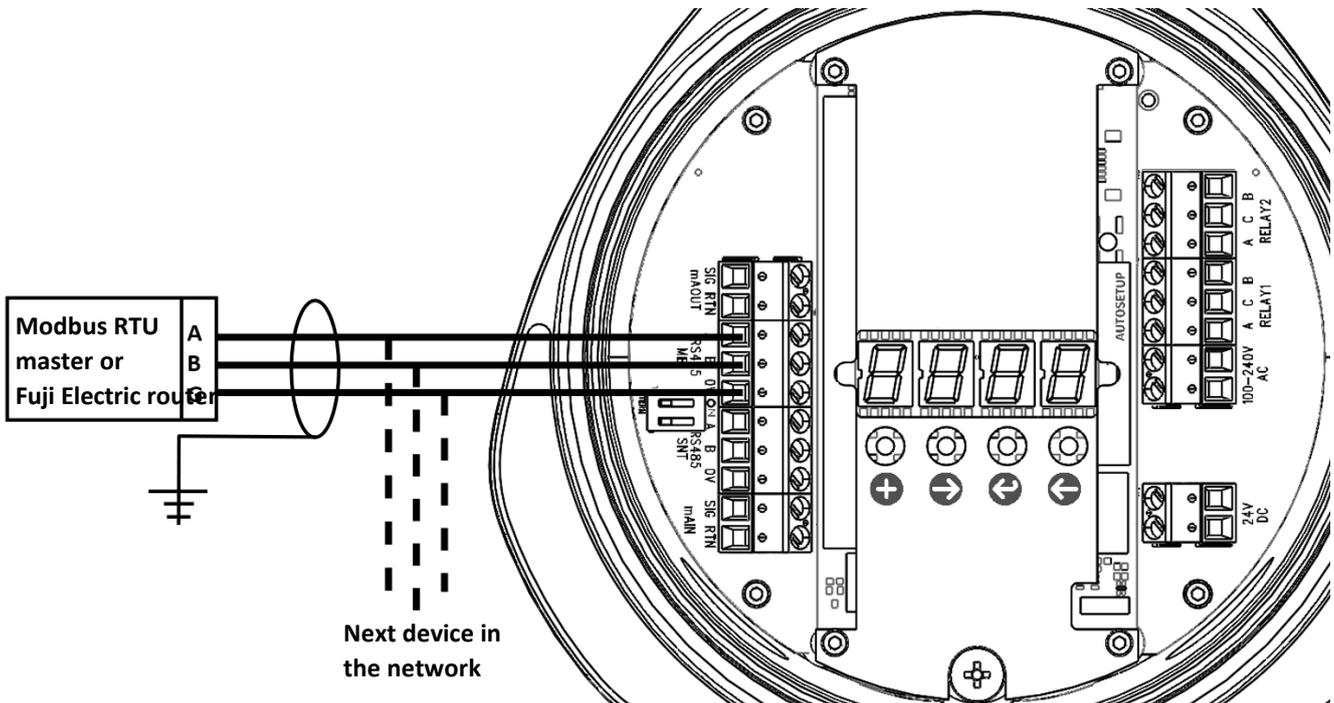
Figure 25: Modbus RTU bus on the main board
