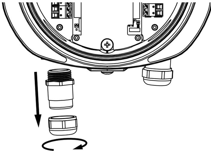
4. Slide the cable gland over the incoming signal cable.
