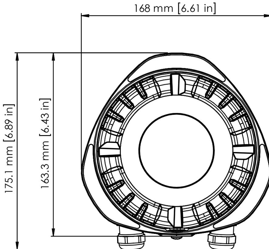
Figure 4: Front view dimensions of the enclosure
