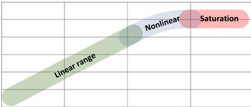
Figure 13: Uncalibrated measuring behavior
