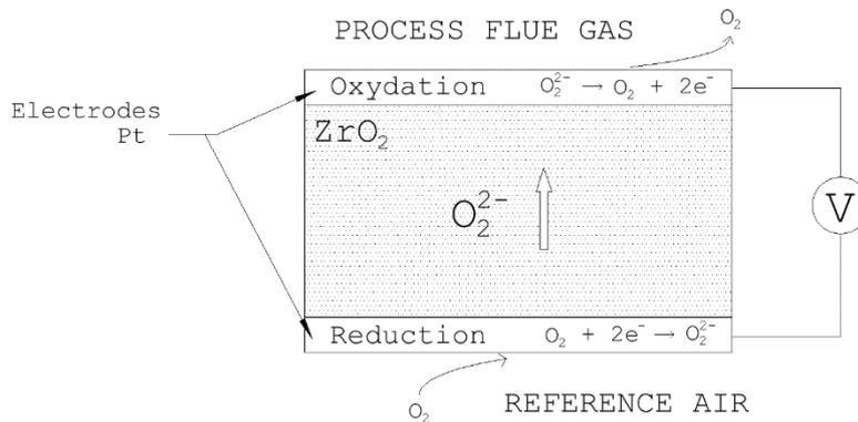
If specimen gas is fed to the outer electrode and a reference gas with a known  $O_2$  concentration, such as air (20.96 %), to the inner electrode, at a constant temperature the logarithmic relationship illustrated below occurs between the probe voltage  $U$  and the oxygen concentration of the specimen gas.
