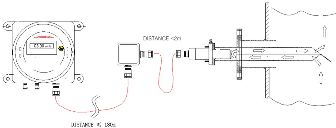
Use Fuji Electric ex-proof compliant cable (red colour) to connect the oxygen transmitter to the junction box. This cable is designed for Fuji Electric analysers:
