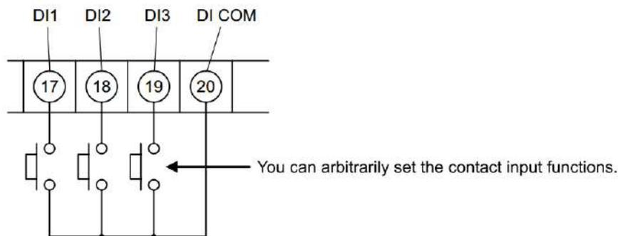
You can arbitrarily set the contact inputs (17) to (19) and (20) of the terminal block.
