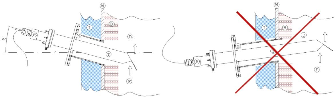
4. If flue gas has to be sampled in parallel to the flow (Angle superior to  $+45^\circ$ ), Fuji Electric provides special deflecting tube with flow boosting system that enable high angle sampling. Please refer to Fuji Electric catalog to get an appropriate deflecting tube regarding your application.
