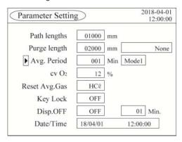
Move the cursor to the "Avg. Period" by using the keys, and then press the key.
