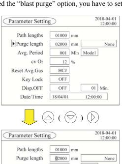
Move the cursor to "Purge Length" by using the keys, and press the key.
