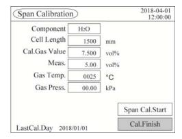
Point the cursor to [Span Cal Start] with and then press (ENT).
