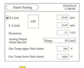
Point the to "H-Limit" or "L-Limit" by the key, and press the key.
