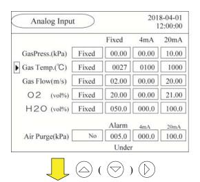
Select the "Gas Temp." by the key or the key. Press the key to move the cursor to "Channel" setting.
