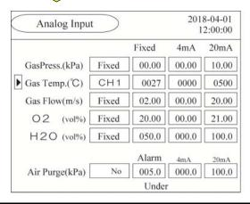
Select the channel (CH1 or CH2) connected to AI terminal by the  $\bigcirc$  key or the  $\bigcirc$  key, and press the  $\stackrel{\text{ENT}}{}$  key.
