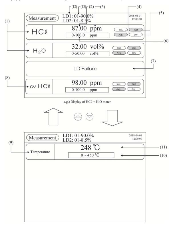
On the measurement screen, the display shows the components being measured, alarm, reference-O<sub>2</sub>-corrected concentration, and analog input. If there are more than four items to be displayed, use UP, DOWN or ENT to move up, down, or across the screen.
