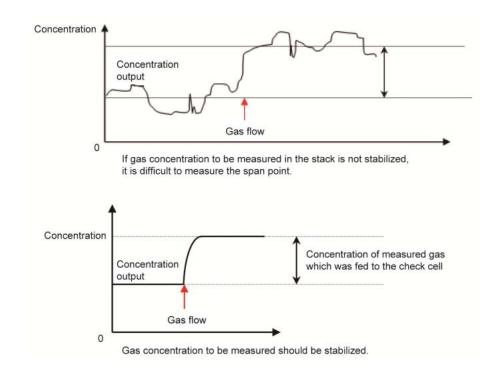
You cannot check the zero point as far as the measured gas exists in the stack.
