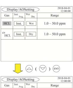
Select the component to be set by the  $\bigcirc$  key or the  $\bigcirc$  key. Press the  $\bigcirc$  key to move the cursor to the "Inst./Avg." setting.
