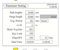
Select "Blast Purge" or "None" by using the keys, and press the ENT key.
