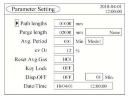
Point the  $\blacktriangleright$  to "Path lengths" by the  $\bigcirc$  key and the  $\bigcirc$  key, and press the  $\bigcirc$  key.
