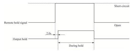
By applying a voltage (pulse width 2.0 seconds or more) to the remote hold input terminal, you can hold the analog output. The hold is cancelled when you stop applying the voltage.
