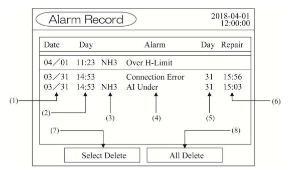
The screen displays the alarm record occurred in the past. The ten newest errors are logged. The oldest error will be deleted one by one every time a new alarm occurs. New errors are displayed from the top on the screen.
