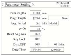
Edit the value by using th keys to change the value, and the key to move to the next digit. Press the ENT key to set the value. (The cursor will move to "Blast Purge".) The "Purge length" setting is completed.
