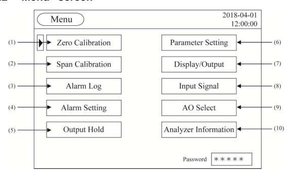
Press the MODE key while the "Measurement" screen is displayed, and the "Menu" screen appears. (It does not appear when pressing the MODE key while other screen is displayed. In that case, Press the ESC key to display the "Measurement" screen, and then press the MODE key.)
