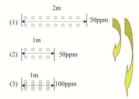
The absorption intensity is twice that of where the gas concentration is 50ppm. and the optical path lengths is 1m.
