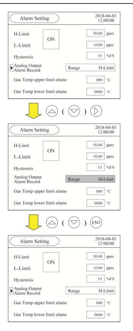
Point the to "Analog Output / Alarm Record" by the key and the key, and press the key.
