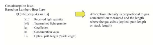
Example: Where the gas concentration is 50ppm and the measured optical path length (stack length) is 2m
