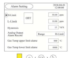
Point the to "H-Limit" to set the H-limit value, and point "L-Limit" to set the L-Limit value, and then press the key.
