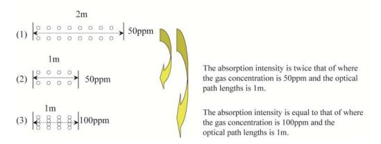
Since the check cell length is 0.25m, the gas concentration to be fed is calculated from the following equation.
