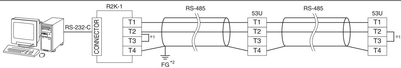
\*1. Internal terminating resistor is used when the device is at the end of a transmission line.
