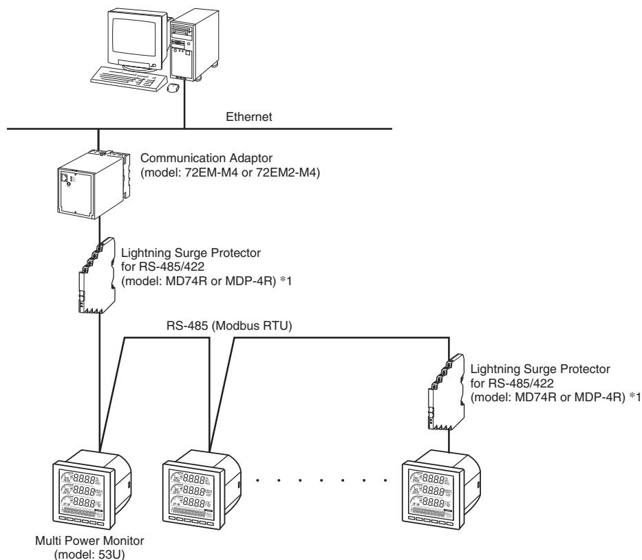
\*1. Insert lightning surge protectors recommended in this example if necessary.
