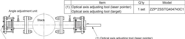
(1) Optical axis adjusting tool (target)
