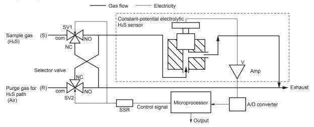
As the H<sub>2</sub>S sensor uses constant-potential electrolytic method, there must be oxygen included in the sample gas. Therefore, air is supplied to the sensor at regular intervals to enable gas analysis in biogas plants where oxygen is absent, and thus stable readings are provided.
