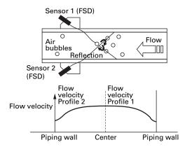
The above shows an example when using two sensors. One detector displays the flow velocity profile for a radius
