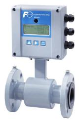
The electromagnetic detector type VI is available with different flange process connections (DIN, ANSI, JIS, AWWA, etc.) and liners like hard rubber or PTFE. Available in sizes from DN 15 to DN 600 and nominal pressures up to PN 100, the detector type VI is best suited for a variety of flow counting applications in the water industry.
