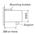
\* 70% or more of the analyzer weight should be supported at the bottom of the case. (In case of mounting panel or 19-inch rack provide a support at the end of casing.)
