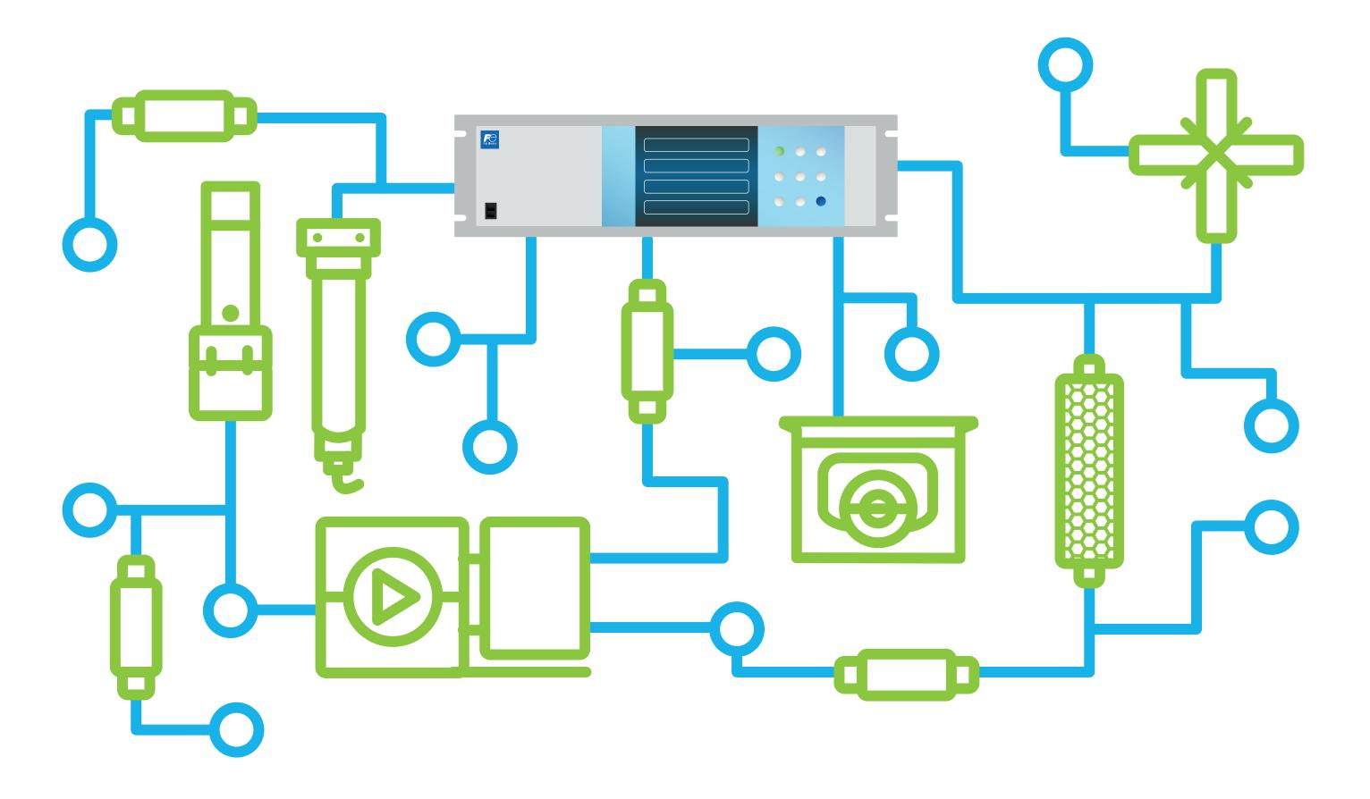
Flame arrestor / drying / filtering / H<sub>2</sub>S scrubbing pressure and flow monitoring / purging
