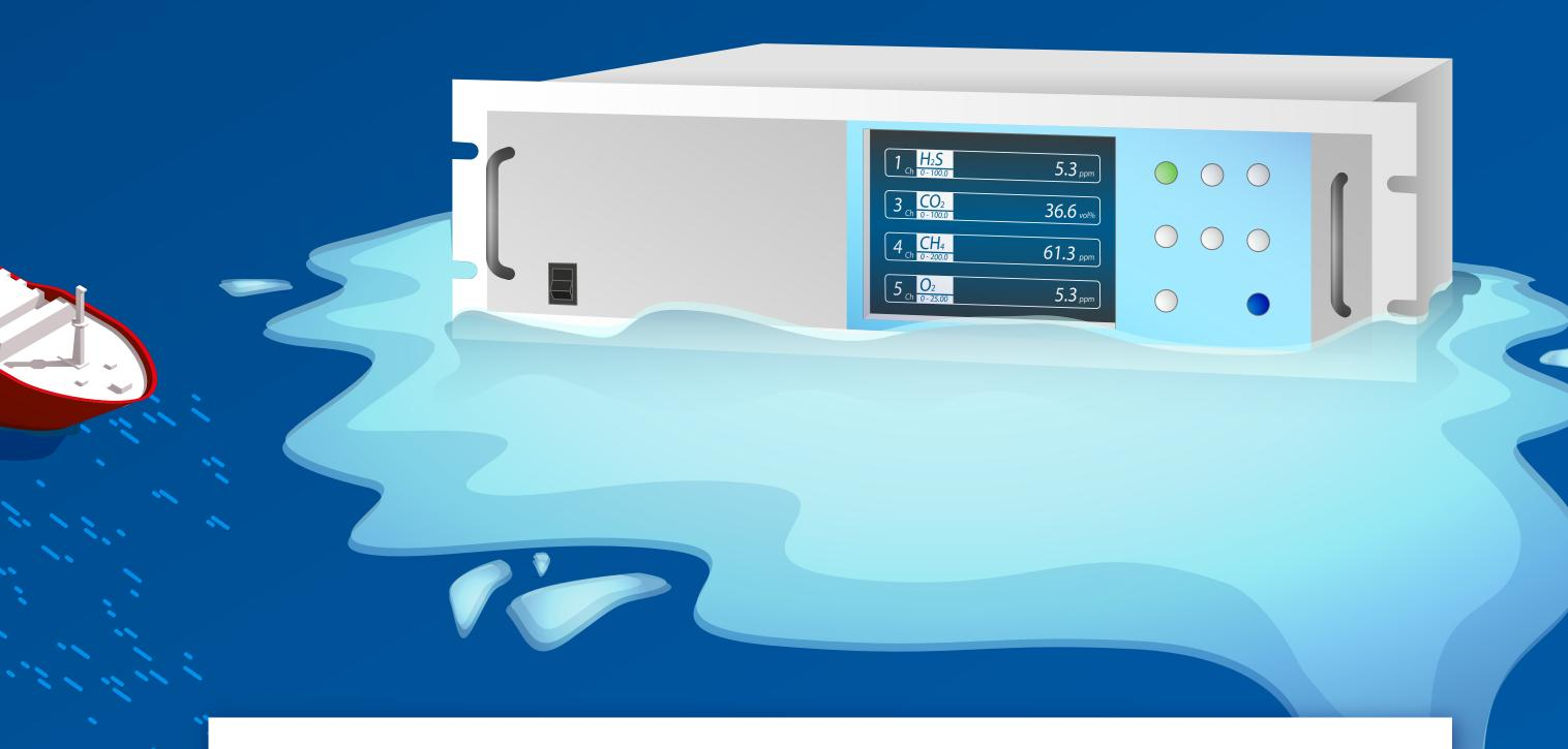
"flooded" analyser with water saturated fumes downstream EGCS
