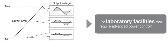
With PWMAPR-M, you can produce a clean sine wave<sup>\*</sup> at any output range (no transformer for tap-switching is needed). \*The output waveform depends on the input waveform. The distortion rate is also affected by input and output. For details, see the "Distortion rate" on page 15.
