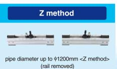
(A detector is simply attached to the exterior of the piping.)
