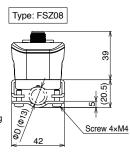
$\Phi$ D: Pipe outer diameter ( $\Phi$ 13- $\Phi$ 18)  $\Phi$ D: Pipe outer diameter ( $\Phi$ 20- $\Phi$ 28)
