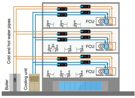
Flow measurement per fan coil unit (FCU)
