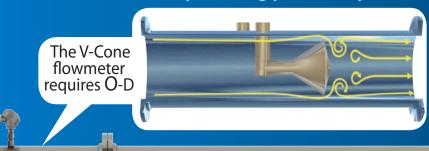
The V-Cone flowmeter acts as its own flow conditioner by disrupting all centralized flow disturbances.
