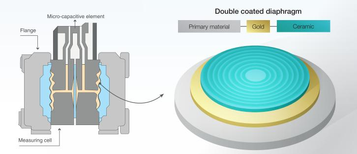
In applications where H+ ions are present, care must be taken to select diaphragm materials that are not susceptible to permeation. All metals show permeability to hydrogen.
