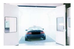
The paint booth is the most energy-intensive part of a car bodywork, accounting for about 75% of total energy consumption. The aim is to use the booth as sparingly as possible in terms of heating and duration of use.
